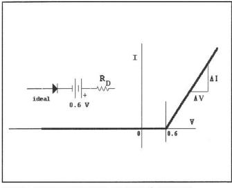
Fig 2.3—IV characteristic for a refined diode model.
