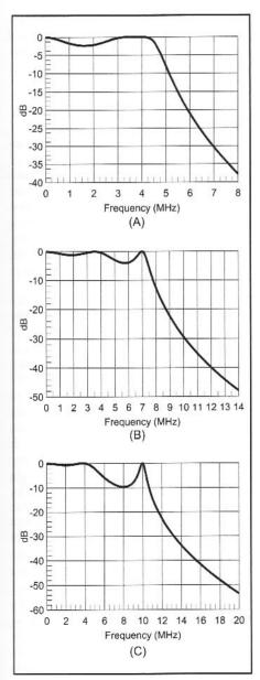
ripples are not necessarily of equal magnitude. The Chebyshev filter is a special case of the ultra-spherical. The transfer function for three variations of the ultra-spherical filter is shown in **Fig 3.8**. All of these 5th-order filters are designed at the highest peak frequency rather than at a cutoff frequency. **Eq 3.1** and **Eq 3.2** still apply. The g(n) values are shown in **Table 3.2**.
