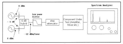
Fig 7.34-Test setup for testing components.
