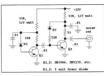
Fig 7.72—Noise in D1 is amplified in a two-stage amplifier, resulting in a strong noise source suitable for measurements. Virtually any diode or transistor types can be used in this source.
