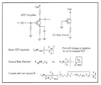
Fig 2.19—JFET bias circuit and equations. The left circuit is a practical amplifier, while that on the right is the bias equivalent. Pick a desired drain current,  $I_D$  (must be less than  $I_{DSS}$ ), and use the middle equation to find the required source resistor. The resulting source voltage is given by Ohm's Law.
