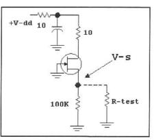
Fig 5.3—Biasing setup for FET modeling.
