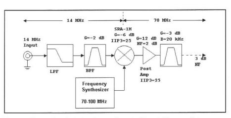
Fig 6.86—Front end typical of modern equipment, although this example is designed for performance beyond the norm. The bandpass filter, shown for 14 MHz center frequency, will have a bandwidth of several MHz and will be switched with relays or PIN diodes. See text.
