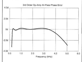
Fig 9.57—Phase errors in the network shown in Fig 9.56. Note the change in scale.
