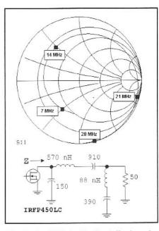
Fig 2.106—50- $\Omega$  Smith chart display of impedance for a 400-W amplifier operating at 13.5 MHz. See text.
