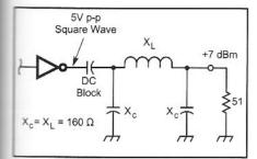
Fig 9.41—CMOS logic with a 5 V supply can drive +7 dBm into diode mixers using this circuit. The pi network converts the high-impedance IC square wave output into a sine wave and transforms the impedance down to drive a  $50-\Omega$  load.
