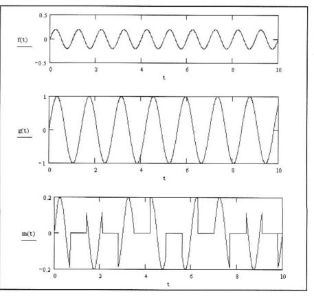
Fig 5.9—Time domain waveforms for a single diode switching mode mixer. The IF output at any instant is the RF input if the LO voltage is positive, but 0 when the LO is 0 or negative.
