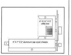
Fig 12.76—A construction sketch of the 14-MHz R2pro.
