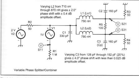
Fig 9.34—A variable phase splitter/combiner network for a 20-meter receiver or exciter. The PSPICE signal generators allow extraction of S11.
