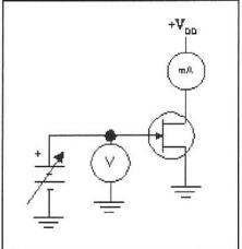
Fig 2.17—Test setup used to evaluate a JFET.
