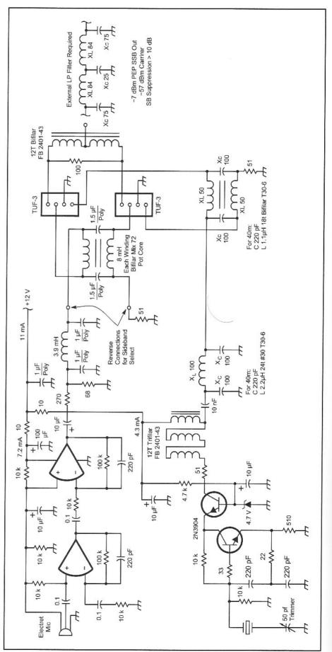
Fig 9.19—A complete schematic of a simple SSB exciter.
