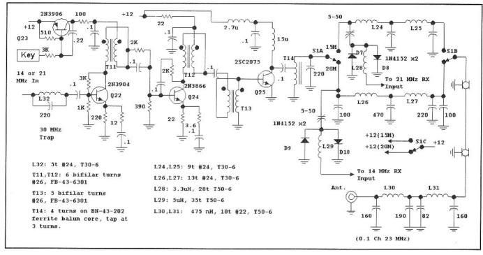
Fig 12.32-RF power chain for the transceiver.
