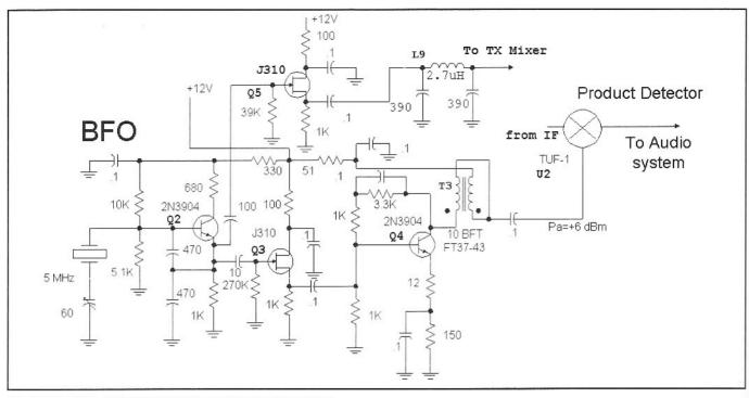
Fig 12.16—BFO and product detector for the Unfinished.
