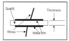
Fig 3.28—Cross section of a quartz crystal.
