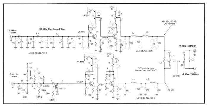
Fig 12.26—The LO signals are processed in this board. The 30-MHz signal is bandpass filtered, amplified, and low pass filtered. The 5-MHz signal is amplified and low pass filtered. Outputs are combined with a 0-degree hybrid. Another hybrid splits the signals, providing +7 dBm for both the transmit and receive mixers.
