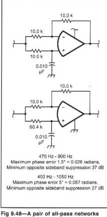
with the 90° frequencies chosen for good suppression over an audio band from 470 to 900 Hz.
