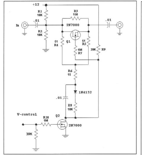
Fig 6.37—A 10-dB pad using electronic switching. A bridged-Tee pad (R3, 4, 5, 6) is switched with low-cost MOSFETs. During thru operation, Q1 is on while Q2 is off. Q2 comes on during attenuated operation. Current consumption is about 1 mA.
