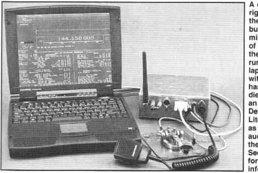
A complete QRP ria for 2-meters. the DSP-10, is built around a minimal amount of hardware and the software running in the laptop PC. Along with the RF hardware in the die-cast box is an Analog **Devices EZ-KIT** Lite that serves as the last IF and audio portions of the transceiver. See page 11.27 for more information.
