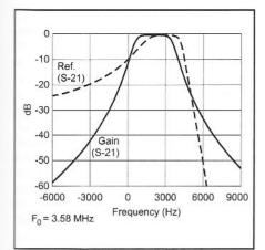
Fig 3.39—The response of two crystal filters built from 3.58-MHz color burst crystals. One uses ideal crystals with zero C0 to produce a symmetrical shape. The other (with dashed line) uses C0=4 pF crystals.
