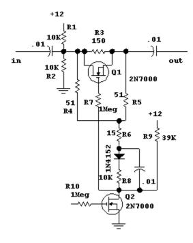
Fig 6.37 (9 Dec 03) Note: The first version of this figure we had on the web was wrong. The "pull-up" resistor to +12 V should go to Q2 rather than to the anode of the diode. The circuit in the 2nd printing of EMRFD is NOT correct. It is still wrong in the
