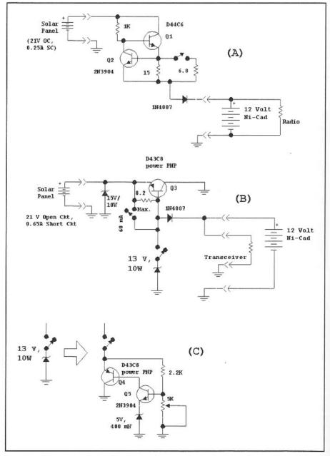
Fig 12.3—Some circuits for handling solar panels. See text for discussion. A TIP-32 may be used for the power PNP, replacing the D43C8.
