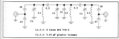
Fig 6.149—Triple-tuned 40-MHz bandpass filter. This circuit was built on a small scrap of circuit board material (approximately 1 × 3 inches) with coaxial connectors mounted at each end. After the filter was tested, a wall was built from %-inch brass sheet and soldered to the board. A lid was soldered to the brass walls after filter tuning. The filter was designed for a 2-MHz bandwidth. The inductors had an unloaded Q of 130 at 40 MHz.
