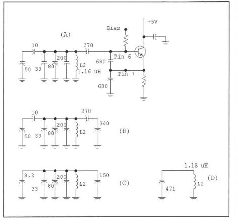
Fig 1.10—Simplified version of the oscillator in a NE602. See text for explanation.
