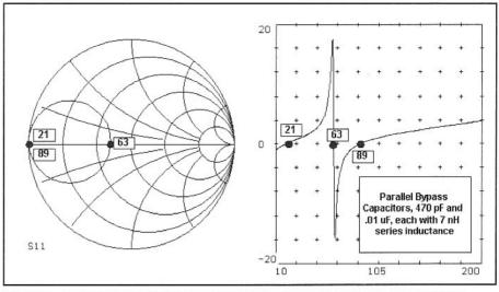
Fig 2.90—The classic technique of paralleling bypass capacitors of two values, here 470 pF and .01  $\mu F.$  This is a terrible bypass! See text.
