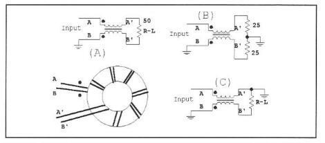
Fig 3.75—Part A: Basic isolation transformer using a transmission line on a ferrite toroid. This structure has some balun like properties. Part B shows a balanced load connected to a single-ended drive while C shows polarity inversion.
