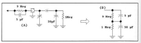
Fig 7.8—A 10X oscilloscope probe. Part A shows the probe and the input to the attached scope while B shows an equivalent circuit. See text.
