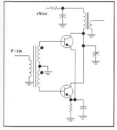
Fig 5.41—Basic push-push frequency doubler using balanced bipolar transistors.
