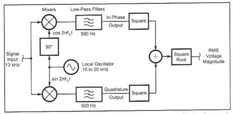
Fig 10.34—An improved implementation of the circuit of Fig 10.33. The in-phase and quadrature outputs will never be zero simultaneously, regardless of the input phase relative to the local oscillator. Blocks have been added to square the in-phase and quadrature outputs, add these together and then take the square root. This produces the RMS voltage of the signal input at the frequency of the local oscillator.
