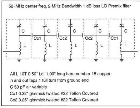
Fig 12.57—Schematic of the 52-MHz premix filter.
