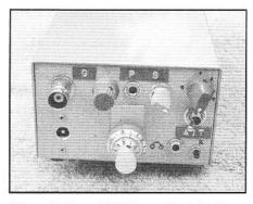
All controls and I/O lines attach to the end of the "Western Mountaineer," allowing it to reside in a small camera case inside a parka. The turns counting dial is on a 10 turn pot to control a temperature compensated VCO. The knob in the upper right corner allows the supply voltage to be "measured."
