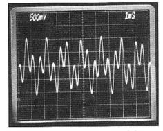
Fig 11.12—Oscilloscope trace of the Audio Generator output. The sinewaves are of equal amplitude and the frequencies are 700 and 1900 Hz. The noise is set to zero.
