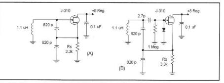
Fig 4.9—Two versions of a Colpitts oscillator. The variation at B is more tolerant of FET variations. The lower noise versions of this oscillator have larger C with reduced L values.
