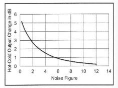
Fig 8.20—Hot-cold resistor noise figure differential.
