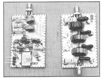
Breadboarded carrier oscillator and TX low-pass filter for a 14-MHz version of the transceiver by K7TAU.
