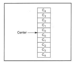
Fig 10.19—Table of FIR filter coefficients for  $N_f$ =10. Only half of the coefficients are calculated and are placed in the second half of the table. The first half of the table is arranged symmetrically as shown. The design program performs these operations automatically. If the number of coefficients is odd, the symmetry remains about the middle coefficient, which must then be doubled in value, since it only occurs once.
