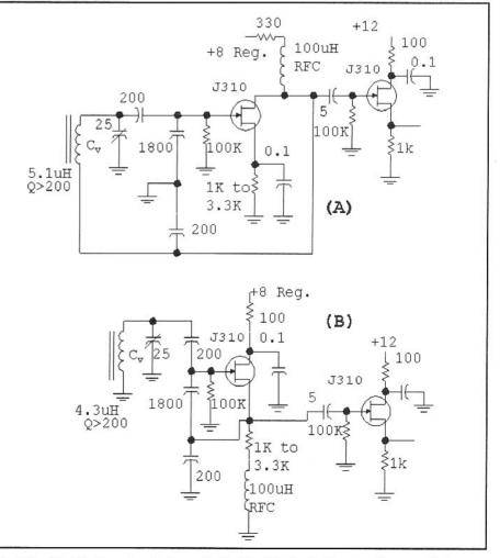
Fig 4.14—The Vackar circuit shown is identical to the Seiler circuit presented earlier except for the choice of component values.
