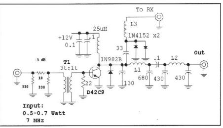
Fig 2.97—High efficiency amplifier after W7EL. T1=3-turn primary, 1-turn secondary, #30 wire, on Fair-Rite 2843002402 Balun core. Count one turn on a balun core as a pass through *both* holes. L1=0.71  $\mu$ H= 13 t. on T44-6; L2= 1.05  $\mu$ H = 19 t on T37-6, L3=15 mH molded RFC. Q is a GE D42C9 plastic power transistor.
