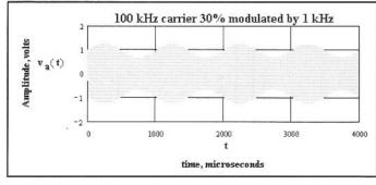
Fig 6.5—The carrier amplitude here is 1 V. Modulation causes the amplitude to depart from this value. The energy appears in the figure to be a solid mass of energy, but if we zoom in, plotting only a small fraction of the curve shown, we will see the details of the RF oscillation. This could be done experimentally with an oscilloscope triggered from the RF waveform.
