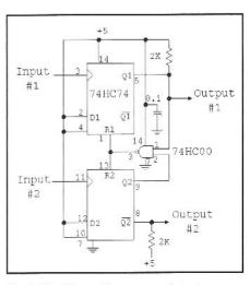
Fig 4.40—Phase frequency detector using digital integrated circuits.
