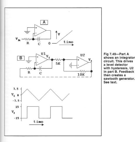
voltage to  $V_{in}$ . This is coupled to the inverting input, which causes U1's output to begin increasing. But this is coupled back to the inverting input through the capacitor. The equilibrium we require of a closed feedback loop in an op-amp is realized when the U1 output voltage ramps linearly upward. The current in the capacitor then equals that in the resistor,  $V_{in}$ /R. Had we applied a positive input we would generate a negative going ramp.
