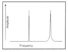
Fig 4.17—A spectrum analyzer output showing two signals with identical amplitude. The peak at the left is "perfect," having a vertical spike shape. The width represents the spectrum analyzer bandwidth. The right hand signal has noise, which appears as a modulation on either side of the carrier. The flat horizontal line is the background noise level of the spectrum analyzer.
