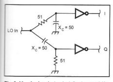
Fig 9.42—A simple logic LO phase-shift network.
