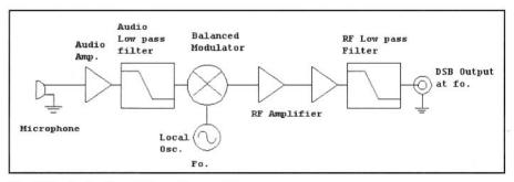
Fig 6.24—A double sideband transmitter.
