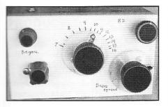
Fig 1.14—Front panel view of the regenerative receiver.
