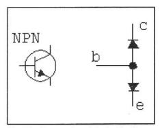
Fig 2.6—Apparent model of a bipolar transistor. This is what we would infer by examination with a VOM.
