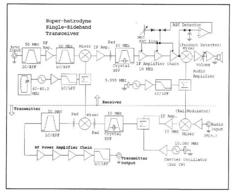
Fig 1.7—Block diagram of a super-heterodyne SSB transceiver.
