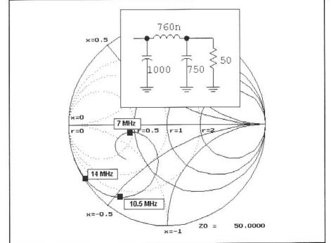
Fig 2.104—Smith chart plot of the impedance "seen" by the collector of the 2N5321 2-W "Beginner's Transmitter" from Chapter 1.
