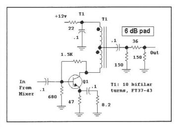
Fig 5.34—Post mixer amplifier using a medium power, high F-t bipolar transistor. See text.
