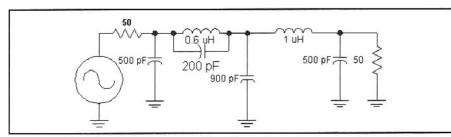
Fig 3.10—Changing an inductor to a "trap" creates a frequency of very high attenuation in the stopband.
