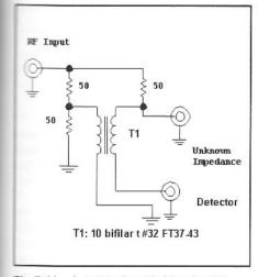
Fig 7.41—A return loss bridge is also known as a 6-dB hybrid. The detector impedance should be 50  $\Omega$  for accurate calibration.
