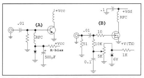
Fig 2.100—Biasing schemes for linear amplifier operation of (A) bipolar transistors and (B) power FETs. The base RFC used with the BJT can have small reactance, for the input impedance is low. The diode is bypassed with a  $500-\mu$ F electrolytic capacitor. The base resistor may or may not be needed. R-bias in (A) should have moderate dissipation, for the current may be high.
