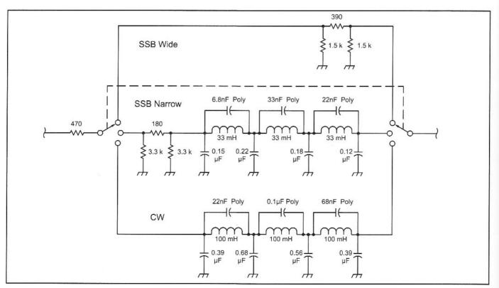
Fig 9.72—A pair of useful audio 500-Ω SSB and CW filters using standard value inductors and capacitors that have been used in a number of our radios.
