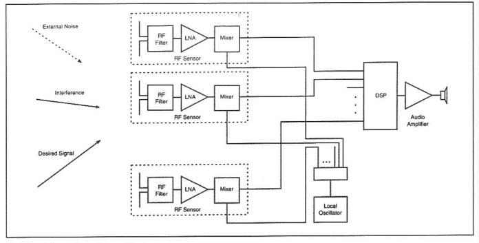
Fig 8.23—Advanced receiver architecture.
