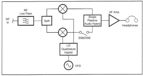
Fig 9.17—Receiver block diagram.
