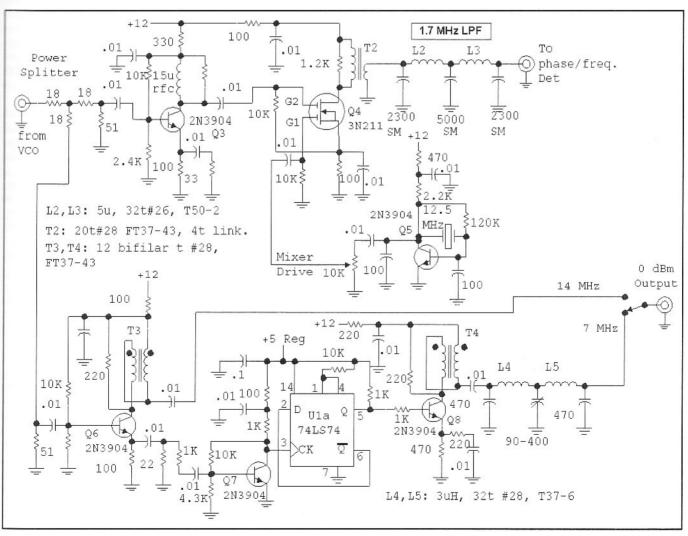
Fig 4.44—Mixer section for the tracking PLL.
