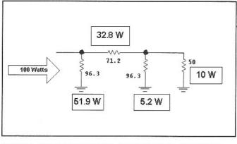
Fig 7.20—Power dissipated in each resistor is shown for a 10-dB pad with 100 W applied. The numbers are also percentages.
