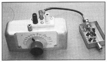
Clean-up gear to reduce the harmonic content of a signal source. This is used when evaluating a transmitter or other source for harmonic distortion.
