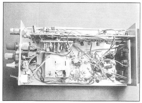
Inside shot of the Western Mountaineer showing the VFO and transmitter, excluding voltage-measuring circuitry.
