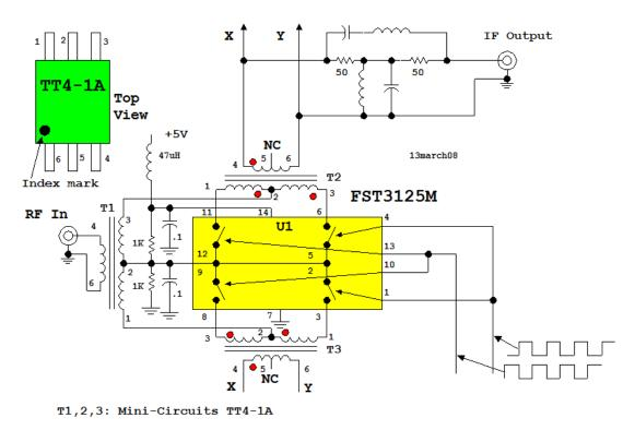
This shows the configuration. I have added some color to make sure that we differentiate this from the earlier drawings. Red phasing dots have also been added to the drawing to emphasize the relationship, not only between the primary and secondary of transformers T2 and T3, but between the two halves of the secondary.
