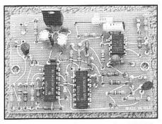
Phase-frequency detector using LS-TTL logic. This circuit is shown in Fig 4.45.
