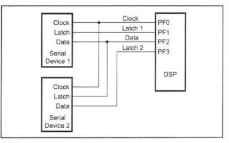
Fig C—Schematic diagram of two serially programmed devices sharing data and clock wires, but having individual latch lines.
