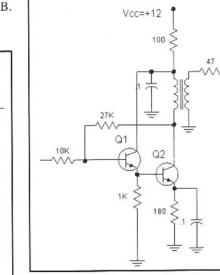
Fig 2.79—Feedback amplifier, the design of W7EL, often used as an oscillator buffer.
