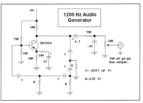
Fig 7.25—A simple audio generator for transmitter testing.
