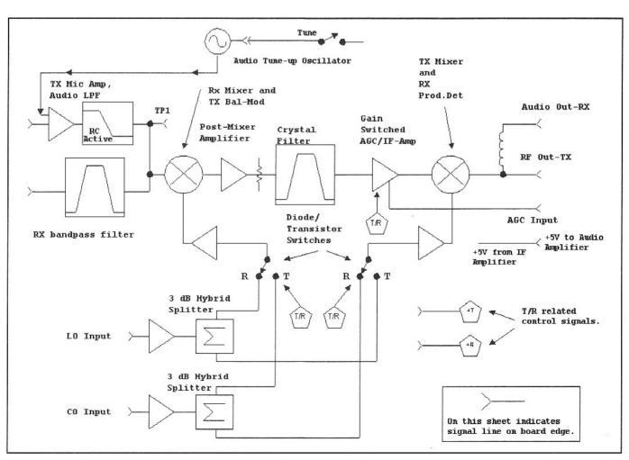
Fig 6.131-Block diagram for the transceiver main board.
