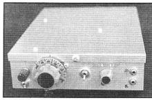
Front panel view of dual band transceiver.
