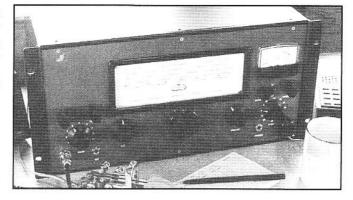
Fig 12.53—The 52-MHz IF transceiver in operation.
