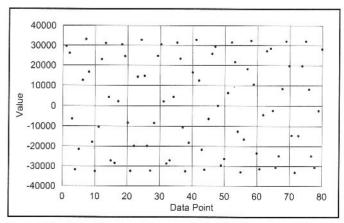
Fig 10.12—Calculated points for a 8500 Hz sine wave. The sample rate is identical with that of **Fig 10.11**. Careful study will show that these are indeed sample points on a sine wave. The ability of the low-pass filter to connect these points into a smooth curve is not so obvious, yet the resulting sine wave is exact.
