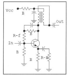
Fig 2.64—A practical feedback amplifier. Components marked with "B" are predominantly for biasing. The 50- $\Omega$ output termination is transformed to 200  $\Omega$  at the collector. A typical transformer is 10 bifilar turns of #28 on a FT-37-43 ferrite toroid. The inductance of one of the two windings should have a reactance of around 250  $\Omega$  at the lowest frequency of operation.
