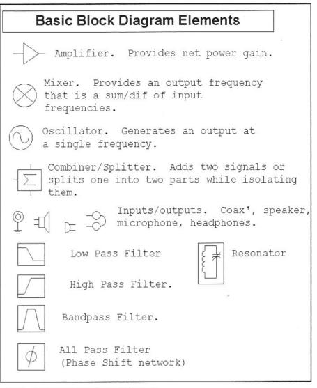
Fig 1.5—Common block diagram elements.
