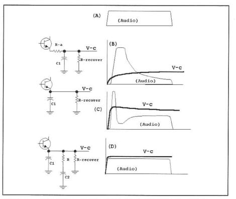
Fig 6.53—Audio envelopes and timing capacitor values vs time. See text for details.
