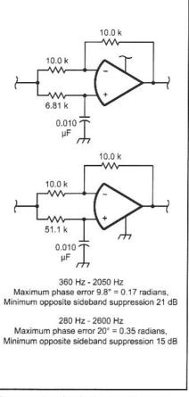
Fig 9.50—A pair of all-pass networks that provide at least 21 dB suppression from 360 to 2050 Hz.
