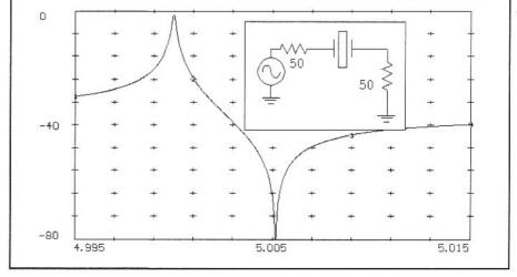
Fig 3.30—Crystal in a 50- $\Omega$  system with response. This crystal has a 5-MHz series resonant frequency, L<sub>m</sub>=.098 H, Q=240,000, and C<sub>0</sub>=5 pF.
