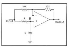
Fig 3.59—Basic, single section all-pass filter. This circuit has unity gain at all frequencies, but has a continually changing phase response. It is useful for phase shift networks such as those used for the phasing method of single sideband.
