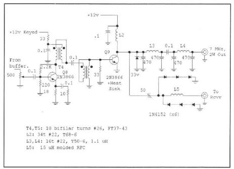
Fig 4.52—Driver and power amplifier portion of the Mk II Ugly Weekender.
