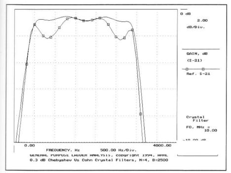
Fig 6.105—Two 4-element crystal filters are compared. The shape marked with small squares represents the Cohn filter while the other was designed for a 0.3 dB Chebyshev response. The two filters have similar skirt response, which is much better than a Butterworth shape, but much worse than a higher-order filter.
