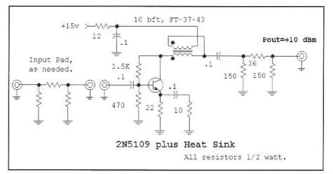
Fig 7.35—Feedback amplifier used following *each* IMD generator to increase the power to +10 dBm per tone. Amplifier gain is 22 dB at 14 MHz, which is reduced to 16 dB with the output pad, Using a 6-dB input pad with the source of Fig 7.8 provides +10 dBm/tone output.
