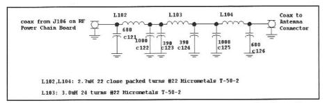
Fig 6.145—Low-pass filter for the 75-meter Lichen. Capacitors can be silver mica or ceramic.
