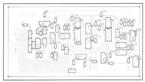
Fig 12.43—View of the component side of the circuit board. Copper runs on both sides of the circuit board are shown. The board layout is double sided, through-hole plated, and was done with the program *Express PCB Version 2.1.1* found at www.expresspcb.com.
