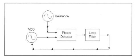
Fig 4.36—Basic Phase Locked Loop.
