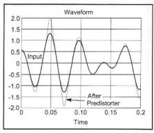
Fig 10.50—Waveforms before and after the predistorter. Only the extreme voltages are increased by the predistorter. This increases the drive to the amplifier to overcome the amplitude compression in the amplifier.
