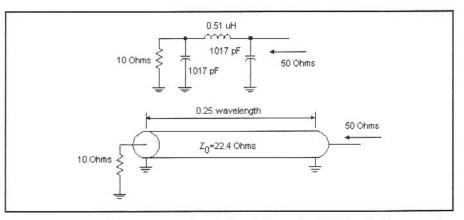
Fig 3.69—A synthetic quarter wavelength line is formed at 7 MHz with three equal reactance values of  $Z_0$  of a Q section.
