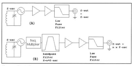
Fig 6.18—Simple CW transmitters with a *master oscillator* and a *power amplifier* are traditionally called a MOPA design. Design "A" has the oscillator and amplifier operating at the same frequency while that at "B" uses frequency multiplication.
