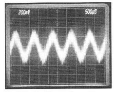
Fig 11.11—Oscilloscope trace of the Audio Generator output. One sine wave is set to 150-mV RMS and the other to zero. The noise level is 50-mV RMS making the S/N 9.5 dB (20\*log(3)). The sine-wave frequency is 1000 Hz.
