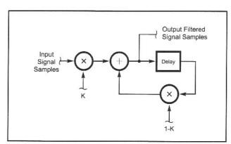
Fig 10.17—Block diagram of the simple IIR filter that has the response of an analog RC low-pass filter. The output signal is delayed by a sample period and a fraction of this is fed back to be summed. This use of feedback is characteristic of IIR filters.
