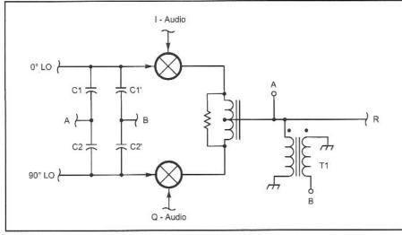
Fig 11.25—Schematic diagram a circuit for increasing L-R isolation of a balanced mixer. In order to minimize the capacitance values, one should never use both C1 and C1' or C2 and C2', as this would only increase the size of both capacitors. All capacitors are a fraction of a pF, made from gimmick wires, which are merely two enamel covered wires twisted together. The transformer, T1, is 5 turns of #26 bifilar wire on a small ferrite core, such as Amidon FT-23-43.
