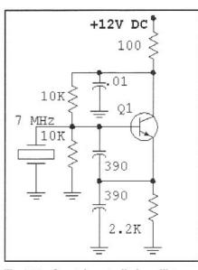
Fig 1.32—Crystal controlled oscillator that is the start of the beginner's transmitter.
