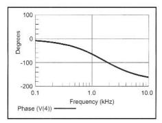
Fig 3.60—Phase response for an all-pass filter.
