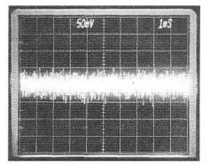
Fig 10.3—Oscilloscope trace of the A/D converter noise in the EZ-Kit Lite. There was no input signal to the converter and the DSP was used to amplify the noise by 100. This was then applied to the D/A converter to produce the trace shown. Each vertical division is 50 millivolts and each horizontal division is 1 millisecond.
