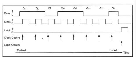
Fig 11.4—Timing diagram for loading the eight-bit 74HC595 shift register with an example binary value of 11011001. Both clocking and latching occur when the signals go from logic 0 to logic 1.
