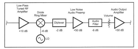
Fig 8.21—A modular receiver block diagram
