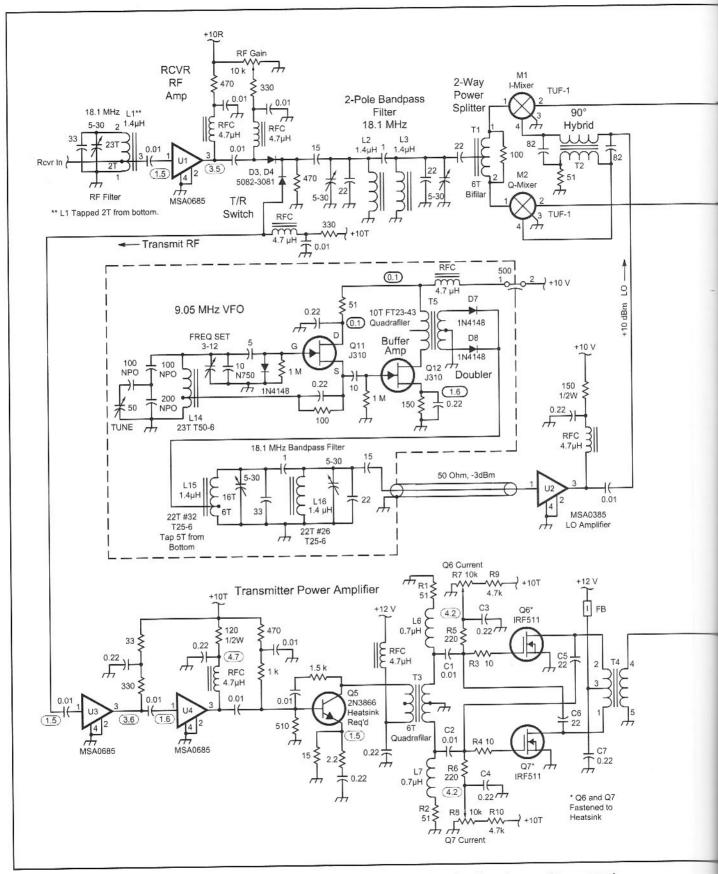
Fig 11.14—Schematic diagram of the hardware used with the 18-MHz transceiver (continued on next two pages).
