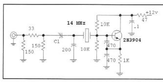
Fig 4.20—Crystal oscillator used for receiver reciprocal mixing measurements. C1 is adjusted for a power output of -10 to -20 dBm.
