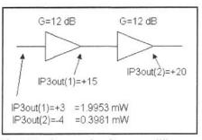
Fig 2.61—A cascade of two amplifiers, each well specified for gain and output intercept. The composite intercept is easily calculated. An extension of this allows an entire system to be analyzed for IMD.
