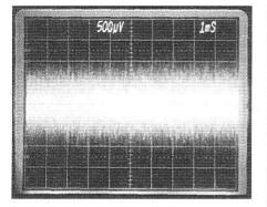
Fig 10.4—Oscilloscope trace of the D/A converter noise in the EZ-Kit Lite. No signal was driving the converter and the oscilloscope bandwidth had been limited to 30 kHz. Each vertical division is 500  $\mu$ V and each horizontal division is 1 mS.
