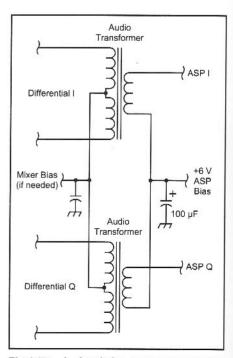
Fig 9.77—A circuit for connecting an I Q balanced mixer output pair into the I and Q inputs of the R2pro analog signal processor board.
