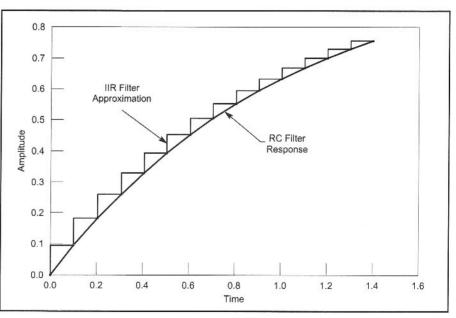
Fig 10.16—The charging response for the RC filter and the IIR filter approximation.
