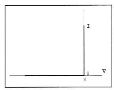
Fig 2.2—IV Characteristics for an ideal or perfect diode. The curve shows I for any possible V that might be applied to the ideal diode.
