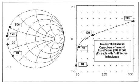
Fig 2.91—Paralleling bypass capacitors of nearly the same value. This results in improved bypassing without complicating resonances.
