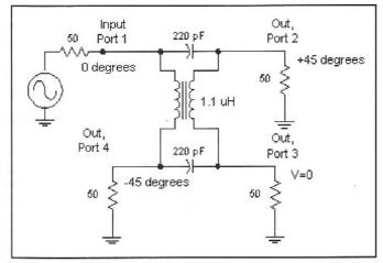
Fig 3.84—Quadrature coupler for 7 MHz.
