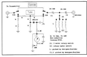
Fig 7.45—Higher power version of a transmatch with a resistive bridge. This unit is rated for 40 W or slightly more for short periods. The topology shown presents a 50- $\Omega$  load to the transmitter while attenuating the signal put on the air by 12 dB. If the resistors specified for R cannot be purchased, parallel combinations of 2-W resistors can be used.
