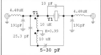
Fig 3.31—A single crystal filter using the crystal of Fig 3-30. T1 is 12 bifilar turns #26 on a FT-50-61 ferrite toroid. This filter has a 3-dB bandwidth of 1.4 kHz.
