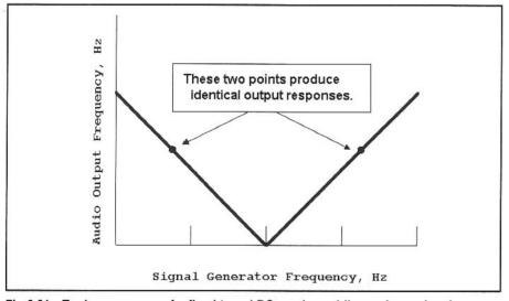
Fig 6.21—Tuning response of a fixed-tuned DC receiver while varying a signal generator applied to the input. A 1000-Hz beat note is available from the generator at two different generator frequencies. One response is the audio image of the other.
