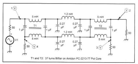
Fig 9.44—A broadband version of the circuit in Fig 9.43 provides marginal performance over a wider bandwidth, but good performance nowhere.
