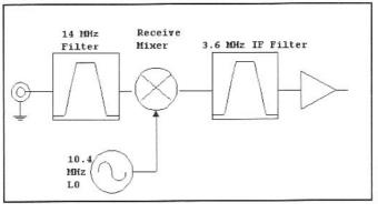
circuits, are illustrated by the system of **Fig 5.11**, a CW receiver for 14 MHz with 10.4-MHz LO and 3.6-MHz IF.
