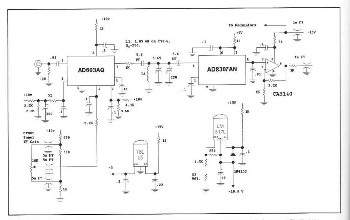
Fig 7.53—This IF and Log Amp section using more accurate integrated circuits and replaces all circuitry of Fig 5 of the original article (see the book CD.) IF gain is variable from 10 to 50 dB. Resistors around the LM317L can be adjusted to set the 10 V level.
