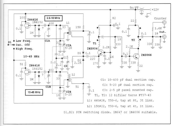
Fig 7.27—General purpose oscillator tuning the range from 3 to 45 MHz in two ranges. See text for details.
