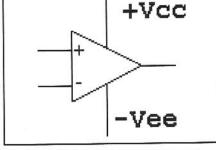
Fig 2.49—Schematic diagram for an operational amplifier.
