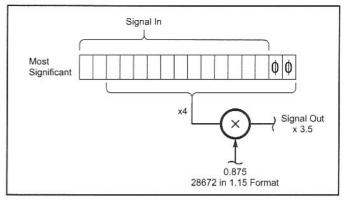
Fig 10.9—DSP gain of 3.5 using a shift register and a multiplier. A gain of 4 is first applied by the shift register, as was done in **Fig 10.8**. Following the shifter, an attenuation of 0.875 is applied, using the multiplier of **Fig 10.7**. This brings the net gain to 3.5.
