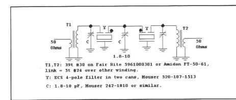
Fig 7.51-4th order monolithic crystal filter.
