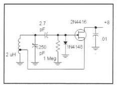
Fig 4.4—Practical 7-MHz Hartley oscillator.
