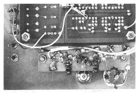
Fig 12.62—Close-up of LO quad-rature hybrid.
