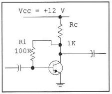
Fig 2.12—Improved bias is obtained from the collector.
