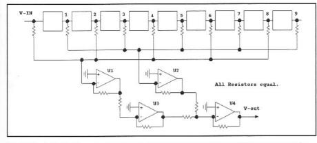
Fig 3.62—A Finite Impulse Response, or FIR bandpass filter built from a cascade of all-pass filters. This filter has 9 taps. Op-amps U1 through U4 serve to add signals from the various taps.
