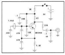
Fig 7.29—Crystal controlled oscillator used for receiver testing. This unit doubles as a spectrum analyzer calibration source with a 7-MHz output of -20 dBm.
