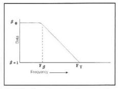
Fig 2.27—Current gain vs Frequency for a BJT.
