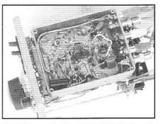
18-MHz transceiver shielded box circuit detail showing extensive use of the "ugly" construction method.
