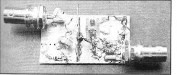
Close up of common-gate low-noise amplifier using a J310.
