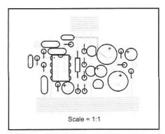
Fig 9.75—Board layout for the audio power amplifier.
