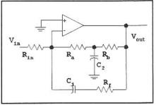
Fig 2.55—The Ra-Rb-C2 network establishes DC bias with little impact on AC gain. C1 and the related resistor then set AC gain. If C1 has a small reactance compared with its series resistor, the gain will grow with increasing frequency.
