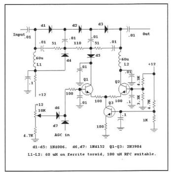
Fig 6.46—IF attenuator circuit offering a 50-dB gain-control range with an insertion loss of about 2 dB at 5 MHz. The 10-kΩ pot is a manual gain control. reduced as signals get larger. The IF in a digital receiver (one where an IF signal is applied to an A-to-D converter) may have more severe requirements related to matching the input signal requirements of the A-to-D.
