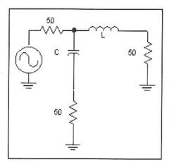
Fig 3.82—First-order low-pass/highpass diplexer.
