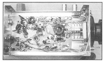
The VFO portion of the transmitter, including diode frequency doubler.
