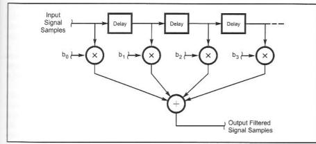
Fig 10.18—Block diagram of the software operations for the FIR filter. The input signal samples are delayed by multiples of the sample period. After multiplication by the filter coefficients, shown here as b<sub>i</sub>, the results are summed to produce the filtered output sample. The output values are not brought back into the calculation as was done with IIR filters. The filter can be extended to the right to increase the performance. Filters with more than 100 coefficients are common.
