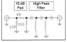
Fig 7.58—High-pass filter used for harmonic measurement. See text.
