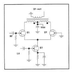
Fig 5.18—A JFET balanced mixer with single ended LO and differential IF ports. This mixer is similar to a bipolar classic, the RCA CA3028A. The RF and LO ports can be interchanged with little performance difference.
