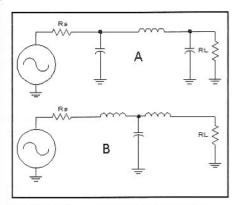
Fig 3.3—Three element, or 3rd-order low-pass filters.
