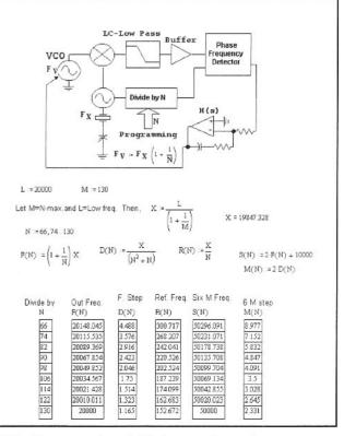
Fig 4.59—Summary of available frequencies and characteristics for a 20-MHz "VXO extender." The result will be frequency doubled where it then serves as the LO for a 50-MHz transceiver based upon a 10.0-MHz IF. This data was generated with MathCad 7.0.
