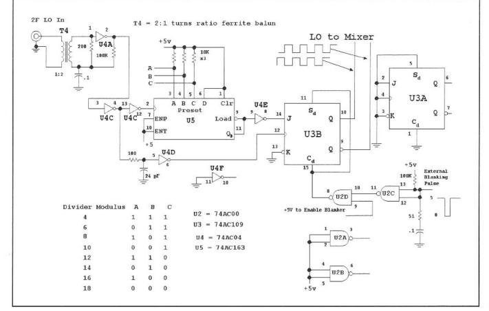
Fig 6.92—Logic circuits accept an input from a VHF synthesizer. The output is then divided by an even number between 4 and 18 before reaching the high-level mixer. The designer/builder must add power supply connections to the ICs.
