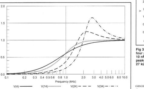
Fig 3.53—Transfer functions for four versions of the high pass section of Fig 3.52. The resistor ratio varies, taking on values of A=1, 2, 5, and 10. The solid line corresponds to A=1 while the highest peak is for A=10.
