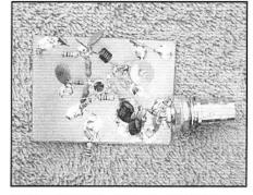
A Butler oscillator. The circuit of Fig 4.28 is breadboarded here without the crystal. Instead, a 51- $\Omega$  resistor is placed in the crystal position. This is a useful way to test the oscillator.
