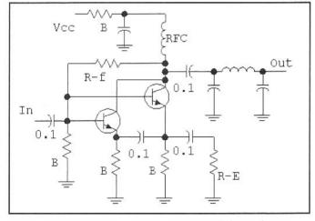
Fig 2.68—Feedback amplifier with two parallel transistors.
