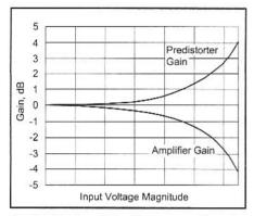
Fig 10.46—Amplifier (lower graph) and predistorter gain characteristics. The two devices are cascaded to result in a net gain that is always 0 dB. The gain of the devices is shown as 0 dB for lowlevels, which is not usually the case and these, should be thought of as relative gains.
