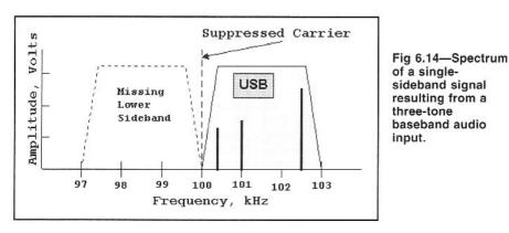
upper and lower sideband components resulting from audio components at  $f_1$ ,  $f_2$ , and  $f_3$ . The DSB signals are shown in **Fig 6.11** and **Fig 6.12**.
