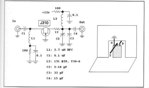
Fig 6.33—A 21-MHz RF amplifier. This circuit, with the values shown, provides a gain of 14 dB with a 5-dB noise figure. Redesign of the input network produced a NF of 1. 5 dB, but with reduced gain of 12 dB. A shield between the source input circuit and the output drain circuit is advised, especially if high-Q solenoid coils are used. It is generally not required when using toroids, although the gate should be grounded with short lead length.
