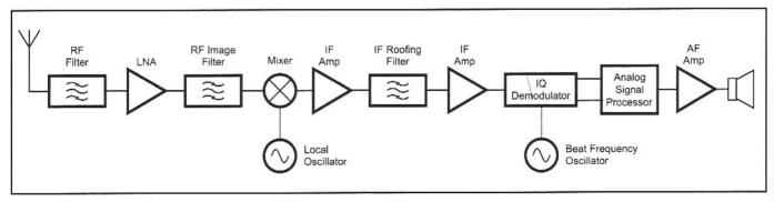
Fig 9.4—A superhet receiver with a phasing SSB demodulator at the IF.
