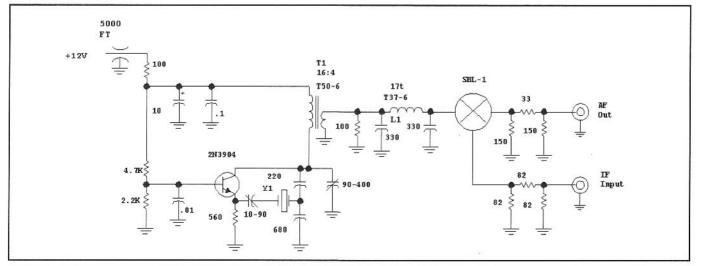
Fig 6.76—BFO and Detector for the 14-MHz receiver.
