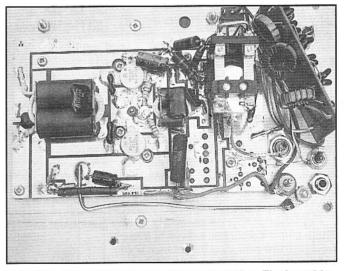
Fig 2.108—Top view of 100-W bipolar amplifier. The board is bolted to a large heat sink that is also the top of the module.
