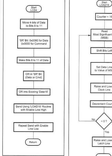
Fig 11.8—Flow diagram for the subroutine Icd4 that transmits 4 bits of data or command to the LCD panel, while not changing the other outputs of the hardware shift register.
