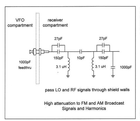
shown in **Fig 12.73**, and the LNA/attenuator is shown in **Fig 12.74**. The 7-MHz RF and LO signals are routed through the shield walls on the feedthrough capacitors using the bandpass networks shown in **Fig 12.75**. This is the best CW transceiver I have ever used.
