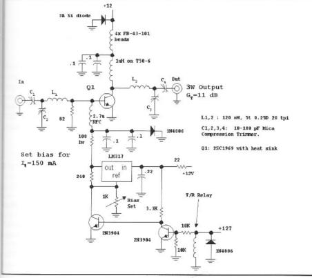
Fig 6.156—A QRP Power amplifier for the 50-MHz band. This circuit is suitable for SSB or CW, and can be adapted to lower frequencies with suitable network changes.
