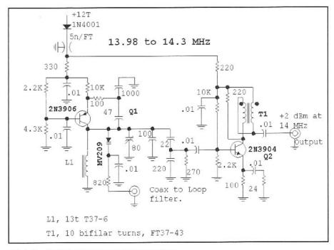
Fig 4.43—VCO for the 14-MHz tracking loop.
