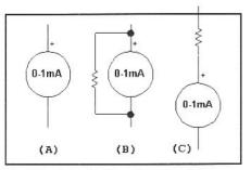
Fig 7.1—A basic 0-1 mA meter (A); measures higher current (B), or voltage (C) with the addition of resistors. Resistance can be measured with these through application of Ohm's Law.
