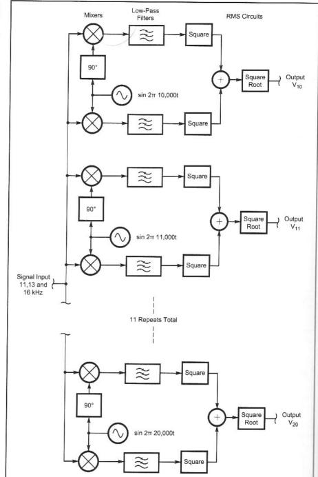
Fig 10.35—A filter bank type of Spectrum Analyzer, built from multiples of the in-phase/quadrature filters of Fig 10.34. As discussed in the text, this structure is equivalent to a Discrete Fourier Transform, followed by the RMS squaring and square-root circuits.
