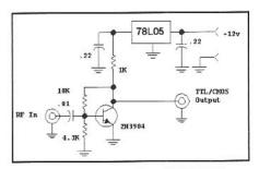
Fig 7.23—Low-level RF to TTL/CMOS converter for simple counting applications. The  $10k\Omega/4.3k\Omega$  resistive divider sets the collector voltage at about 3 times the 0.7 V emitter-base offset, guaranteeing bias in the active region.
