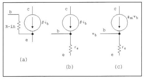
Fig 2.9 Evolution of a small signal transistor model.
