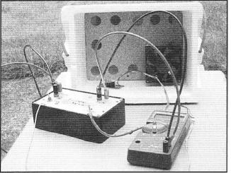
Control box, DVM, and environmental chamber" for oscillator testing. The chamber has the lid removed so an oscillator can be placed inside. The lid is then place on the box. A light bulb heater resides under the press wood base with holes. A 12-V fan moves the air within the box. Cables to the oscillator under test and the IC used for temperature measurement are routed under the lid edge.
