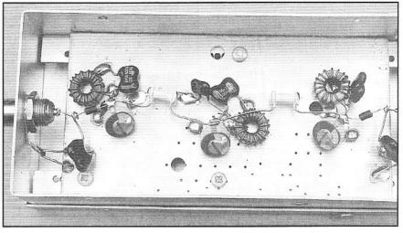
Fig A—Bad filter—This bandpass filter performed well around the 7-MHz passband but had poor stopband attenuation. A very deep attenuation notch appeared at about 15 MHz.
