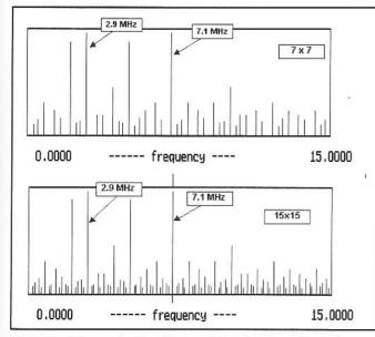
Fig 5.14—Mixer outputs with a variety of orders allowed, n and m to 7 in the upper curve and 15 in the lower.
