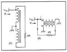
Fig 3.76—A 4:1 step-up balun transformer.
