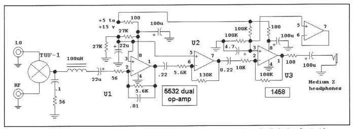
Fig 6.29—A basic direct-conversion receiver. An audio amplifier with a gain of 87 dB follows the diode ring. See text for discussion.
