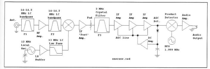
Fig 6.59-14-MHz receiver with a 2-MHz IF. The LO tunes from 12 to 12.2 MHz, so the image extends from 9.8 to 10 MHz.
