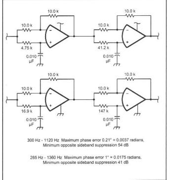
Fig 9.52—A second-order all-pass network pair for CW receivers that provides more than 50 dB of opposite sideband suppression from 300 Hz to 1120 Hz.
