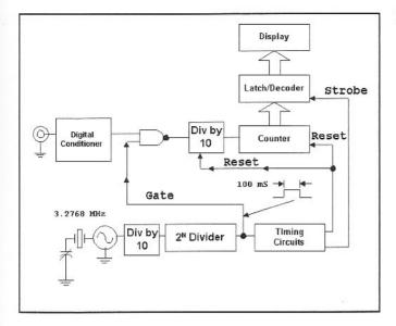
Fig 4.53—Block diagram for counter.
