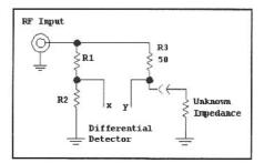
Fig 7.37—A basic bridge circuit.
