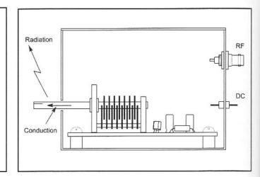
Fig 8.18—Capacitor shaft pickup in an LO box.
