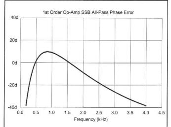
Fig 9.51—Phase errors from 0 to 4 kHz. The errors may be reduced by adding more sections and recalculating the allpass network frequencies.
