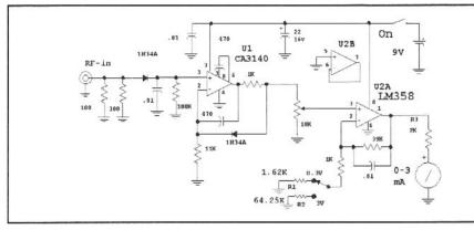
Fig 7.11—This power meter, based on the work of W7EL, has full scale readings of 0.3 and 3 volts RMS with sensitivity of less than –10 dBm. The circuit can be adapted to other ranges. R3 can be changed to 6 k $\Omega$  if a 0-1 mA movement is used. See text for details.
