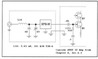
Fig 12.28—Input section of the crystal filter and IF amplifier for the transceiver. See text.
