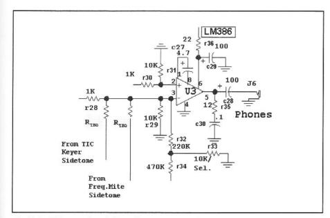
Fig 12.8—Sidetone signals from the counter and the keyer may be injected as shown. Removing R23 will disable the original sidetone from the output.
