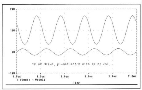
Fig 2.37—Collector (upper) and output load (lower) voltages with the pi network output circuitry.
