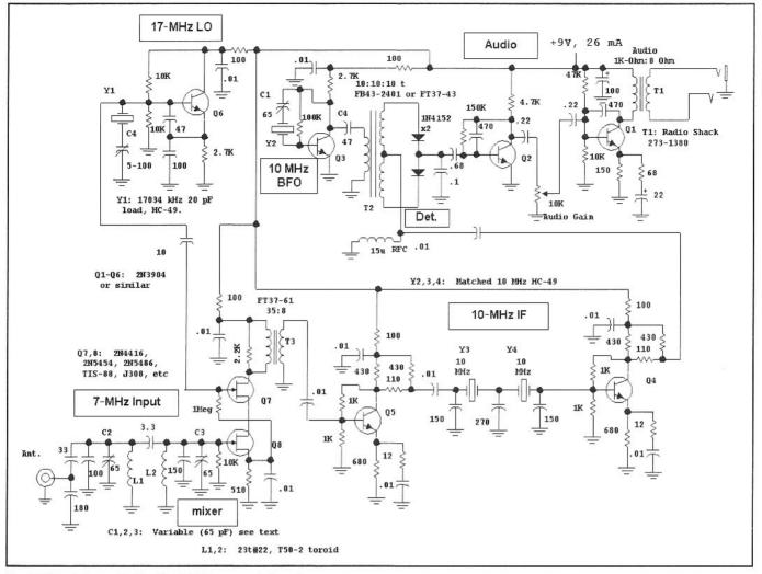
Fig 12.21—Schematic for the 7-MHz super-heterodyne.
