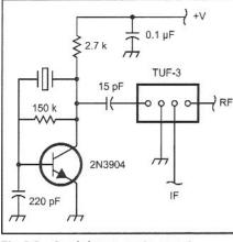
Fig 9.9—A minimum-parts-count frequency converter.
