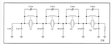
Fig 3.41—Experimental crystal filter. Y1,2,3,4 = 3.58-MHz surplus color burst crystals. ( $L_m$ =0.117H,  $C_0$ =4 pF) L = 151 µH, 48 turns #30 on FT-50-61 Ferrite toroid.(Amidon) C-trim = 3-12 pF ceramic trimmer. See the referenced *QEX* paper for adjustment procedure.
