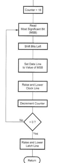
Fig 11.9—Flow diagram of the subroutine load16. This transfers 16 bits of data the hardware shift registers.
