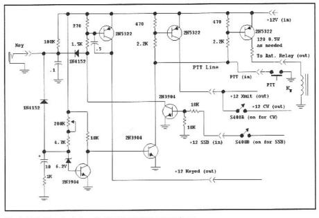
Fig 6.157-Control circuits for the SSB transceiver.
