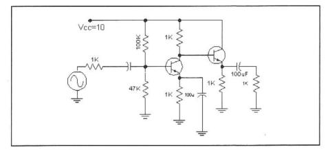
Fig 2.23—Voltage Amplifier with a DC coupled emitter follower.
