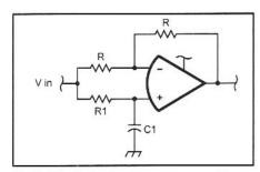
Fig 9.47—A single-stage op-amp allpass network.
