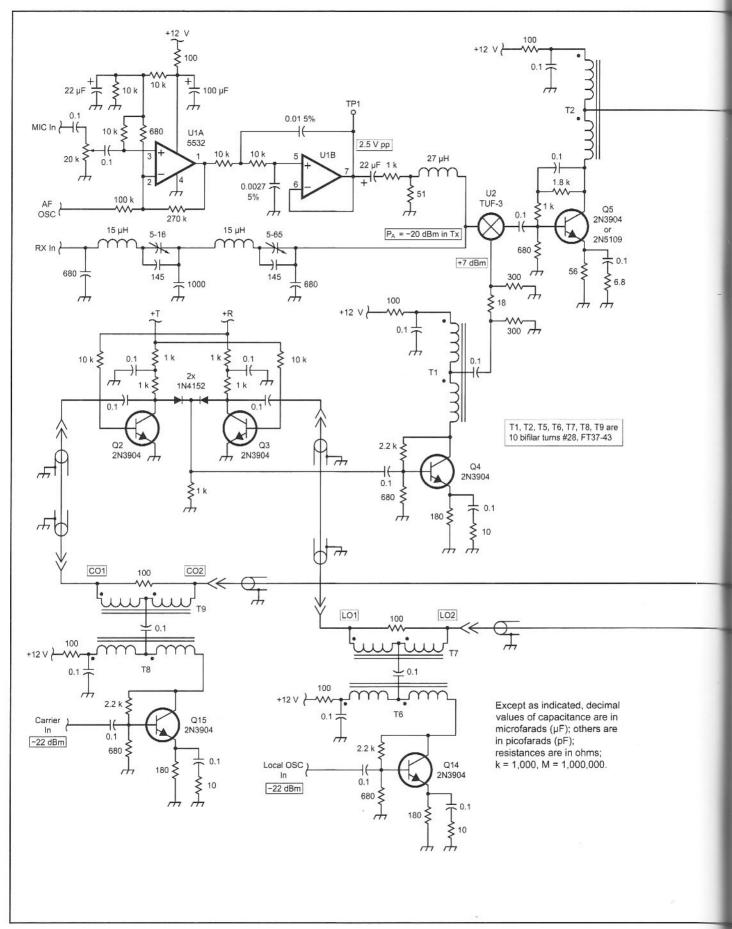
Fig 6.132—Schematic for the main board. See text for detailed discussion.
