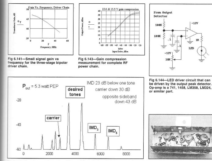
Fig 6.142—Spectrum analyzer view of transmitter output under two-tone testing. For software, see www.monumental.com/rshorne/gramdl.html.
