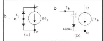
Fig 2.8—A current source is added to the diode pair to form a representative model. The diode is often ignored as in B.
