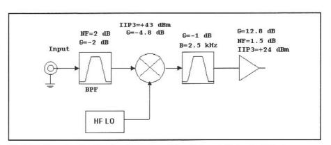
Fig 6.89—Receiver front end using no amplifiers before initial selectivity is obtained. This is the basis of the W7AAZ/W4ZCB/G3SBI receiver described below.
