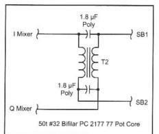
Fig 9.43—This simple quadrature hybrid circuit has good performance at only one audio frequency, but it is truly elegant in its simplicity and provides trivial sideband switching, draws no current, and offers the possibility of binaural independent sideband listening.
