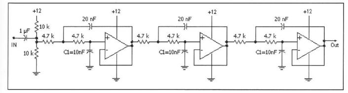
Fig 3.50-Practical low-pass filter that can be built with common op-amps, such as the 741, 1458, 358, 324, 5532.
