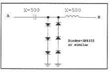
Fig 6.125—T/R switch with shunt PN diodes.
