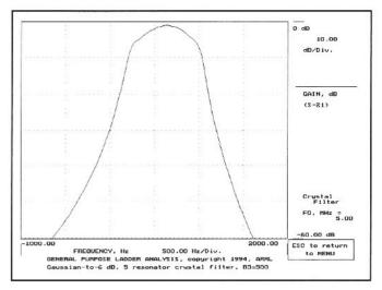
Fig 6.71—Calculated response for the Gaussian-to-6-dB crystal filter. The shape is Gaussian for the top 6 dB, but then reverts to a Chebyshev-like skirt response. The k and q data for this filter were obtained from Zverev's *Handbook of Filter Synthesis*, Wiley, 1967.
