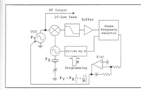
Fig 4.48—A simple PLL synthesizer featuring frequency steps much smaller than the reference frequency.
