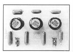
Fig 9.73-SSB and CW filters.
