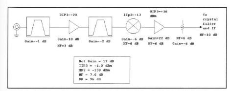
Fig 6.67—An RF amplifier is added to the basic diode-ring front end, significantly improving noise figure while compromising DR by only 2 dB.
