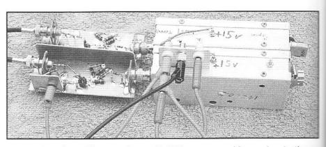
Outside view of matching crystal controlled RF sources used for receiver testing. The outboard amplifiers provide the higher signals needed for testing mixers and high-level amplifiers.
