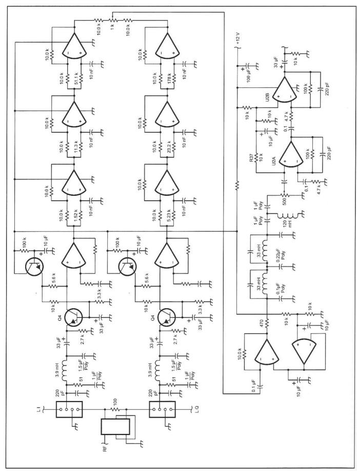
Fig 9.62—This simplified version of the mini R2 uses some different parts values and requires matching of the diplexer components.
