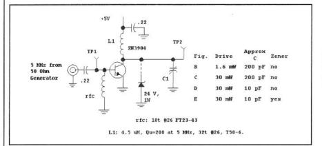
Fig A—RF Drive is applied to the base of a BJT while the un-terminated collector is biased through a tuned circuit. The data table relates results to operating conditions.
