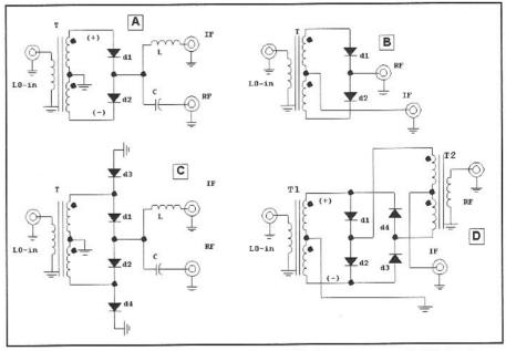
Fig 5.19—Evolution of diode mixers. Parts A and B show narrow and wideband versions of a two-diode mixer. The mixer is expanded to 4 diodes in part C, a circuit offering a better termination for the LO generator. These evolve into a diode ring, doubly balanced mixer in part D.
