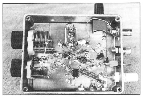
Fig 1.11—Direct conversion receiver assembly.
