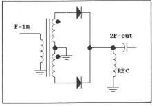
Fig 5.40—Diode frequency doubler. The diodes, ideally identical, can be siliconswitching types, such as the 1N4152 or 1N918 for use at HF and low VHF. Hot carrier diodes are recommended for UHF applications, or for critical, low phase noise HF applications. The transformer can be the familiar 10 trifilar turns on a FT37-43 core for HF applications. Often, this doubler drives a link on a single tuned circuit, eliminating the need for the RFC.
