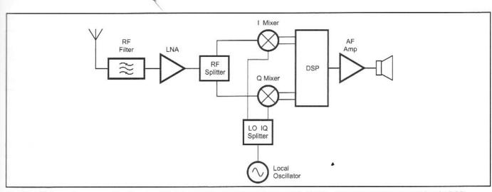
Fig 9.6—High performance direct conversion receiver technique with phasing added—with baseband processing in DSP.
