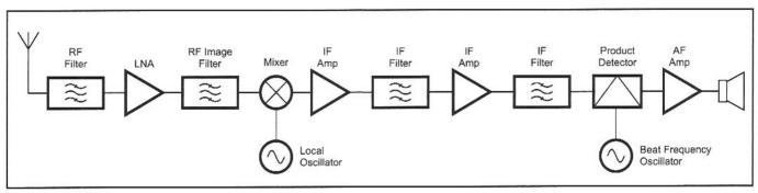
Fig 9.3—A conventional superhet receiver with a SSB bandwidth IF.
