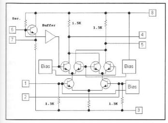
Fig 5.26—Equivalent circuit of the Phillips NE602/NE612.8
