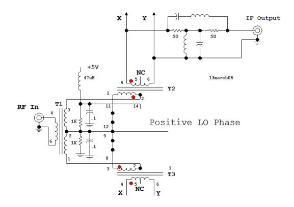
The right switches are open, so are not parts of the circuit at this instant in time. Moreover, we have eliminated the transformer halves connected to them, for no current flows in those windings at that point in time. We can now use this diagram to trace the path between the RF transformer and the IF output and show that the phase relationship is additive for the two current components reaching the IF load. A similar diagram for the negative LO phase can also be generated.
