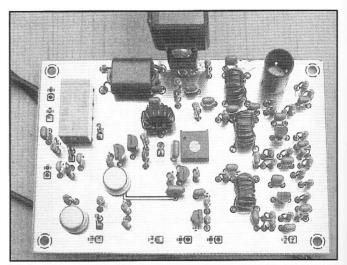
Printed Circuit Version of RF Power Chain. (TNX to K7TAU)
