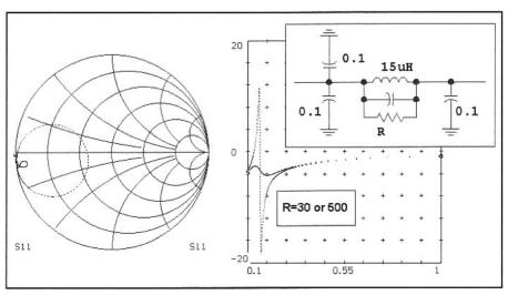
Fig 2.92—Two different resistor values parallel a decoupling choke. The lower,  $30-\Omega$  value is more effective. See text.
