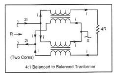
Fig 3.80—A 4:1 balanced-to-balanced transformer.
