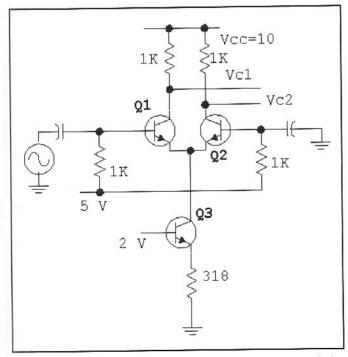
Fig 2.47—Differential Amplifier that converts a single ended signal into a differential one having two outputs with a differential relationship. The 2 and 5-V points are fixed voltage, usually generated within the IC containing this differential pair.
