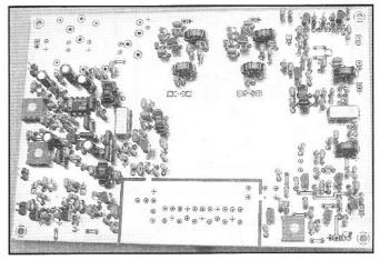
Partially built printed main board.
