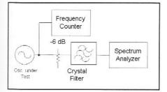
Fig 4.19—System used to measure phase noise in the K7HFD oscillator.
