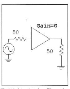
Fig 2.56—A terminated amplifier used for noise analysis.
