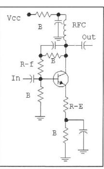
Fig 2.65—A variation of the feedback amplifier with a 50- $\Omega$  output termination at the collector.
