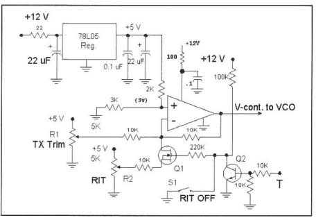
Fig 6.118—Circuitry to control RIT. Q1 is a TO-92 N-Channel MOSFET such as a 2N7000 or VN-10 or Zetex ZVNL-110A. Q2 = 2N3904 or similar. R1 sets the control voltage during transmit. The SPST switch is closed when the RIT is off. In this state, the control voltage should be approximately 7.5 V. The control voltage should vary between 4 and 10 with RIT on. Op-amp type is not critical; it could be a 741, half of a 5532 or 358, or similar.
