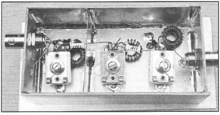
Fig B—Good filter—A box built from scraps of circuit board material produced a response with good stopband attenuation.
