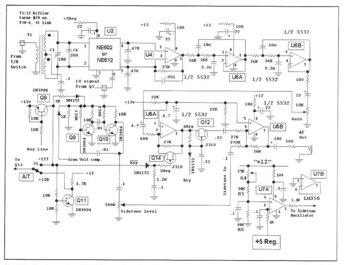
Fig 12.10-Receiver portion of the "Western Mountaineer" transceiver.
