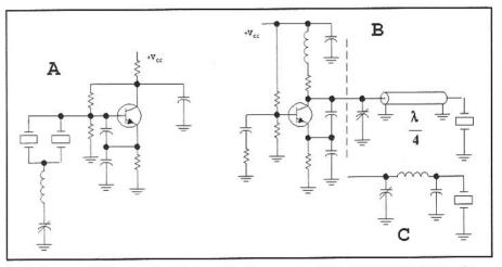
Fig 4.32—Two VXO circuits of interest to the experimenter. That at A is known in Japan as the Super VXO, and is the creation of JAØAS and JH1FCZ. The circuit at B uses a quarter wavelength of transmission line while that a C is the lumped element equivalent.
