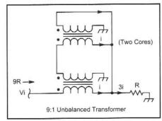
Fig 3.79—Illustration of a 9:1 unbalanced transformer.
