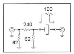
Fig 3.34—Simple test set for crystal measurement. The pad is a 20-dB,  $50-\Omega$  circuit. The output should be terminated in 50  $\Omega$ . A maximum input power from the generator would be about -10 dBm, resulting in a maximum to the crystal of -30 dBm. The 100- $\Omega$  pot is substituted for the crystal for ESR measurement. See text. Approximate equations for motional parameters are:
