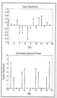
Fig 10.38—This diagram shows (A) 16member time waveform and the power for the DFT output. To emphasize the discrete nature of the data involved, the values are shown as dots with attached vertical lines. Note that the spectral power is symmetrical about the 8th output.
