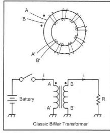
Fig 3.73—Current flow in a bifilar wound transformer.
