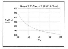
Fig 2.74—Output resistance depends on the source resistance.
