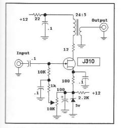
Fig 6.43—A single JFET is biased toward pinchoff with the reverse bias developed across the Zener diode. This amplifier offers 13.5 dB gain and a 37-dB gain range. The transformer, wound on an FT37-43, was available on the bench at the time of testing. The 10-k $\Omega$  pot sets gain.
