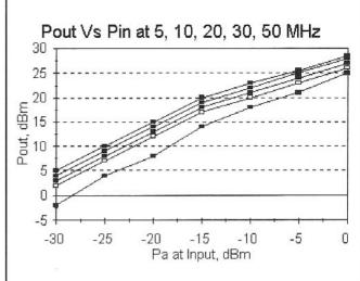
Fig 2.94—Gain compression characteristics for the simple power chain.
