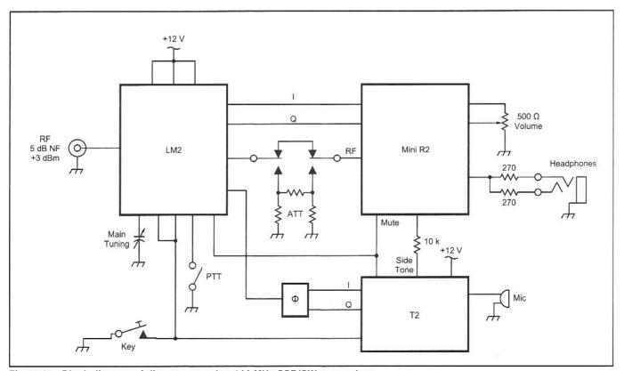
Fig 12.45—Block diagram of direct-conversion 144-MHz SSB/CW transceiver.
