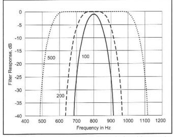
Fig 10.23—Response of three FIR filters designed for a center frequency of 800 Hz, using 200 coefficients and a sampling rate of 9600 Hz. The –6 dB bandwidth was designed to be 100, 200 and 500 Hz.
