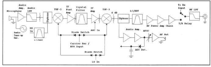
Fig 6.130-Block diagram for the Lichen transceiver.
