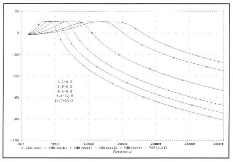
Fig 9.65-LNA swept frequency plot.
