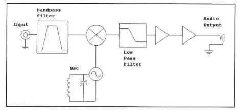
Fig 6.20—Direct-conversion receiver. The incoming signal is applied to a mixer where it is converted directly to audio without intermediate processing.
