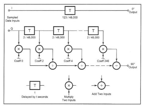
Fig 11.20—Block diagram of the Hilbert transform with 247 taps. The blocks marked 'T' are delays of multiples of sample periods, as indicated on the diagram. Each sample period is 1/48,000 second.
