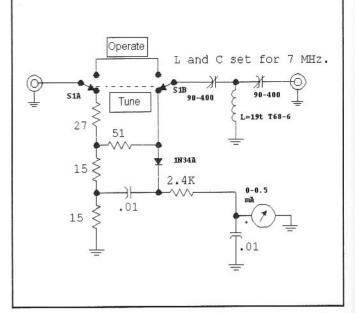
Fig 7.44—7 MHz transmatch and resistive bridge for portable operation. Variable capacitors are screwdriver adjusted, mica compression types. All resistors are 1/2 W. S1 is a DPDT slide or toggle switch. This design is suitable for transmitters up to about 3 W if the tuning is done quickly.
