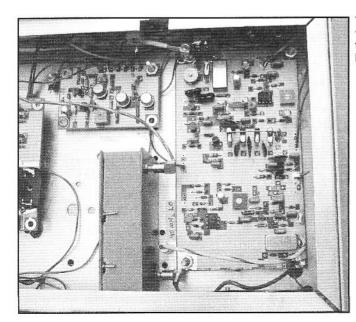
The large board is the SSB generator and transmit mixer. This version used SBL-1 mixers. The transmit bandpass filter is in the box fabricated from scrap circuit board material. The control board is above the bandpass filter.
