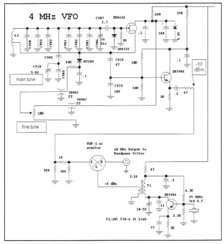
Fig 6.148—VFO for the 6-m transceiver. L1 is unspecified, but will generally be around 5  $\mu$ H. The many resonator capacitors allow flexibility in setting the frequency. Details are set by the designer/builder.
