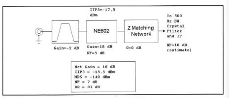
Fig 6.64—A simple receiver/front end using the NE602. The IF system is estimated to have a noise figure of 10 dB.
