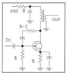
Fig 2.77—A feedback amplifier using a FET. See text for design details.
