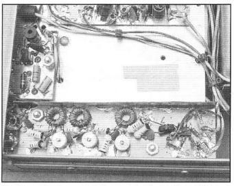
The transmit mixer and triple tuned bandpass filter. Shield strip along one side of the board helps to confine ground currents.
