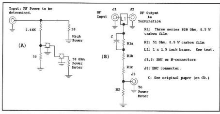
Fig 7.14—Power tap with 40-dB attenuation. Part A shows the basic concept while B shows the version built. See text and original paper on the book CD.
