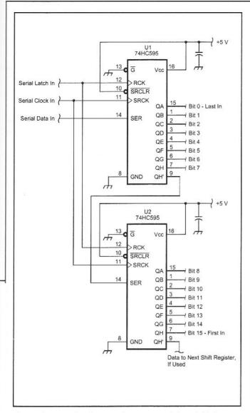
Fig A—Schematic diagram of two cascaded serial-in/ parallel-out shift registers providing 16 logic level outputs.
