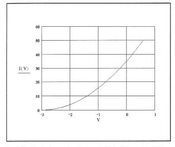
Fig 2.18—Drain Current vs Source-to-Gate Voltage for J310 type Junction Field Effect Transistor.  $I_{dss}$ =35 mA and  $V_p$ =-3 V.  $V_p$  is the voltage where drain current goes to zero.  $I_{dss}$  is the drain current when the gate and source are both at the same potential.
