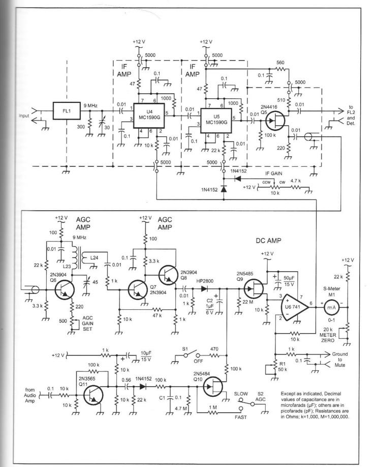
Fig 6.57—A full hang-type AGC system with two timing systems. The IF-derived AGC offers quick attack while "hang time" is established by the audio.
