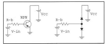
Fig 2.7—The circuit we used to bias a bipolar transistor for active operation. See text.
