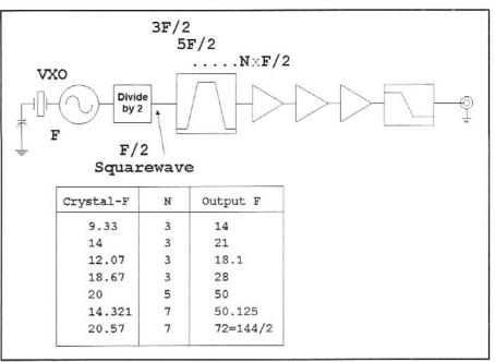
Fig 5.48—Block diagram showing the transmitter concept. The table shows some possible applications.
