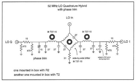
Fig 12.61—Schematic of the 52-MHz LO quadrature hybrid.
