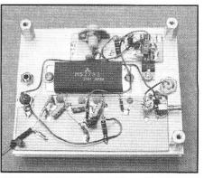
View of RF power amplifier using the Mitsubishi Hybrid. Output is up to 14 W.
