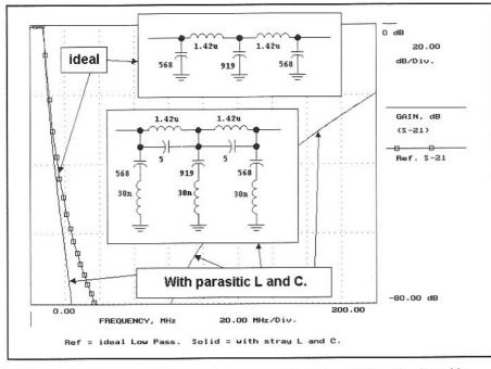
Fig 3.11—The VHF performance of HF low-pass filters is significantly altered by parasitic inductance and capacitance. The parasitic elements are modeled as being larger than normal to illustrate the effects.
