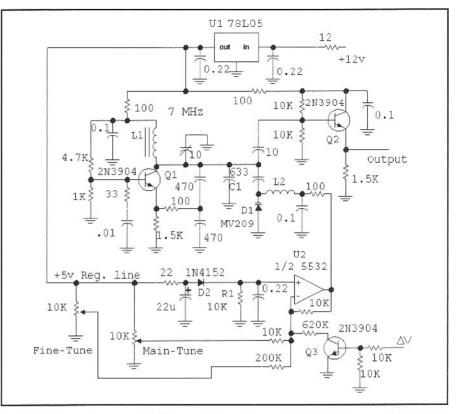
Fig 4.33—A varactor tuned 7-MHz oscillator with a restricted tuning range of about 60 kHz. Temperature compensation is provided with D2, a sense diode. L1=12 turns #26 on a T30-6 toroid. L2 is a 15- $\mu$ H RF choke.
