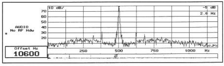
Fig 7.63—High resolution spectrum of a signal generator. The noise is phase noise on the generator. 120-Hz hum modulation is readily observed as well.
