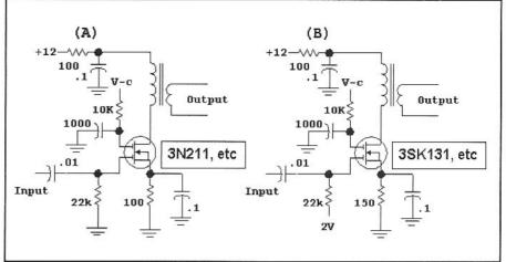
Fig 6.44—Two variations of a basic dual-gate MOSFET amplifier with variable gain. The circuit at (B) has the larger gain variation. The labeling of FETs is arbitrary, for these circuits are intended to be generic. The 3SK131, an SMT device from NEC is popular and is recommended.
