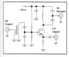
Fig 5.7—Simple bipolar mixer.
