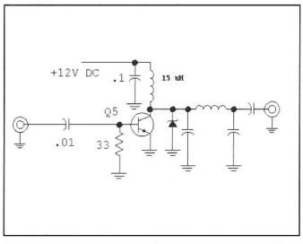
Fig 1.36—Earlier simplified PA design which suffered with stability problems. See text for discussion.
