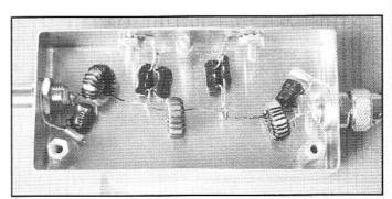
Fig 1.38—Inside view of the 7-element low pass filter built to go with the beginner's rig. The filter is also used with other equipment.
