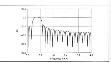
Fig 10.20—Response Curve for a 50-coefficient FIR filter designed to pass 400 to 800 Hz with an 8-kHz sample rate. No windowing function was used with a resulting high out-of-band response.
