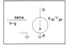
Fig 2.20—Simplified small signal JFET model.
