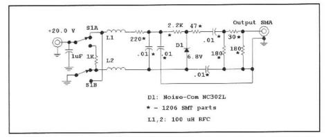
Fig 7.73—Noise source providing a flat frequency response over a wide bandwidth. Our source was built with surface-mounted components where possible. The diode was purchased from Noise Com, East 64 Midland Ave, Paramus, NJ 07652; tel 201-261-8797.
