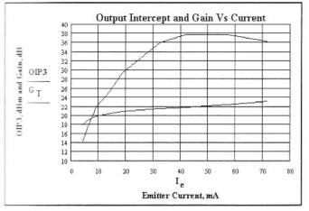
Fig 6.70—Gain (lower curve) and output intercept for one or two 2N3904s in parallel. Two devices should be used for currents above 20 mA, while total current over 40 mA is not recommended except as an experiment.
