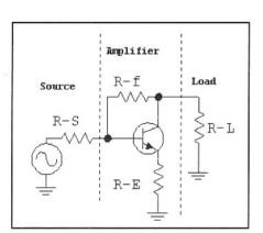
Fig 2.63—Small signal circuit for a feedback amplifier.
