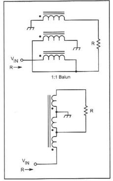
Fig 3.78—A 1:1 impedance ratio true balun transformer.
