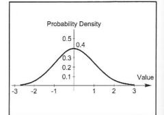
Fig 10.13—Gaussian noise probability curve, showing relative probability of being in the vicinity of any value. The curve extends forever on either side of the graph, but the probability of achieving these values rapidly becomes insignificant.
