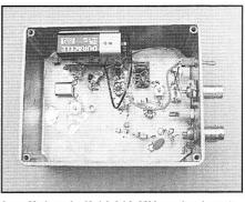
An off-the-shelf 14.318 MHz color burst crystal becomes a convenient RF source for the 50-MHz band. Built by KA7EXM.
