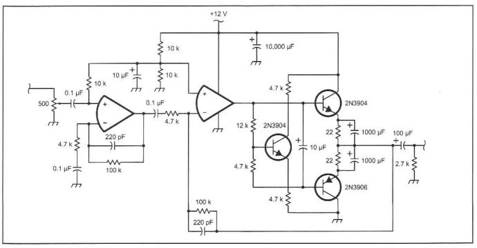
Fig 9.74—An audio power amplifier circuit.
