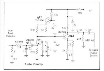
Fig 12.18—Audio preamplifier for the Unfinished.
