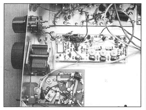
Inside view of the 10-meter module with the VXO and triple tuned bandpass filter in the center. The receiver RF amplifier board is at the bottom of the photo.
