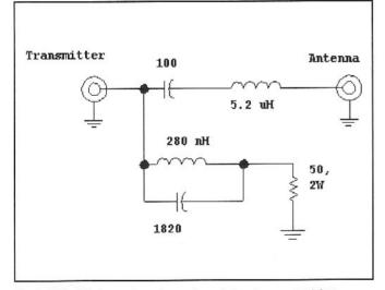
Fig 2.107—Diplexer, bandpass-bandstop type, used for harmonic attenuation from a 7-MHz transmitter. The reader should consult the original *QST* article<sup>23</sup> for details.
