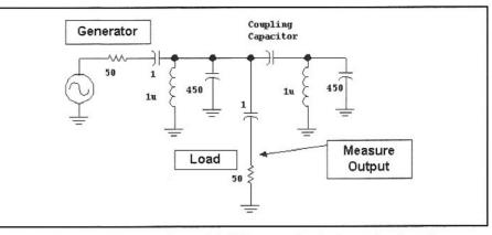
Fig 3.19—Scheme for measuring and defining coupling between two tuned circuits. C12 is either 10 or 20 pF while the resonators are both  $1\mu$ H paralleled with 450 pF. "Probe" capacitors are 1 pF.
