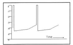
Fig 4.5—Squeeging in a Hartley oscillator, an on-and-off mode where the oscillator is not functioning except during short periods. The vertical scale shows the gate voltage. Extreme values of blocking capacitor and bias resistor are required to produce this behavior in the FET Hartley oscillators.
