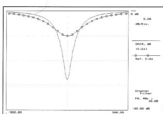
Fig 7.71—Sweeping two crystals while investigating their properties as traps. One has a Q of 40,000 while the one producing the deeper notch has a Q of 200,000. Notch depth is measured to determine Q.
