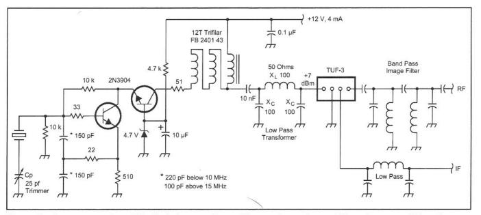
Fig 9.8—If voltages are not sinusoidal, simple low-pass filters will remove harmonics, and if impedances are different from 50  $\Omega$ , transformers may be used. This technique results in receivers with very predictable performance, and many parts. A conservative frequency converter using this approach is shown here.
