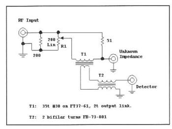
Fig 7.38—RF bridge for HF measurements. R1 is ideally a 100- $\Omega$  linear pot, but all we had was 200  $\Omega$ . The Clarostat 1/2-inch diameter conductive plastic parts should offer reasonable performance, although we have not used them in this application.
