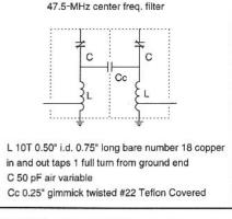
Fig 12.58—The 47.5-MHz premix oscillator filter.
