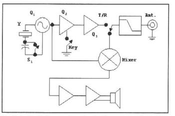
Fig 12.4—Block diagram for a simple direct conversion transceiver. A single crystal oscillator serves a dual function.
