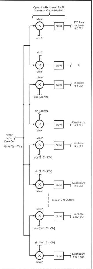
Terminology for the DFT differs from that used for hardware. Our block diagram of Fig 10.35 is in the latter term. Restructured in conventional DFT terminology, Fig 10.36 shows the same filter bank implementation. The RMS voltage blocks have been removed to show only the DFT.
