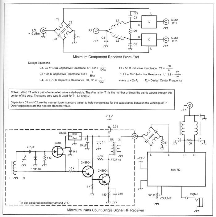
Fig 9.38— A good combination of LO quadrature network and RF splitter for HF and low VHF single-band receivers and exciters.
