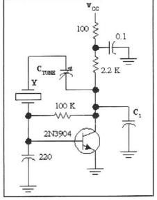
Fig 4.25—Pierce type crystal oscillator. C1 can be as little as 10 to 20 pF. Vcc can be from about 3 up to 15 V.  $C_{TUNE}$ , often omitted, is a trimmer with a maximum of 50 or 100 pF.
