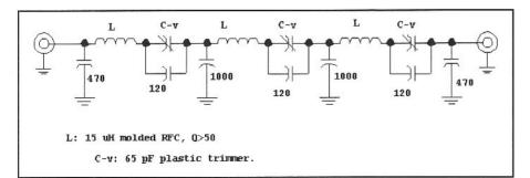
Fig 6.134—Triple-tuned 3.5 to 4-MHz bandpass filter for the output of the transmit mixer.
