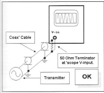
Fig 7.15—Power is measured with an oscilloscope and a 50- $\Omega$  terminator at the scope input connector.
