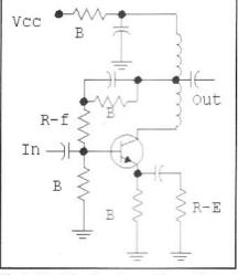
Fig 2.67—A feedback amplifier with feedback from the output transformer tap. This is common, but can produce unstable results.
