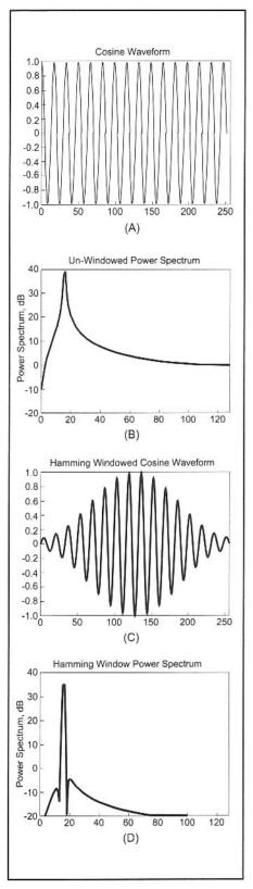
Fig 10.43—Illustrating the use of windowing to minimize spectral leakage, the figures show (a) a cosine waveform, chosen to not meet up at the endpoints, (b) the resulting unwindowed DFT power spectrum, (c) the same cosine waveform with a Hamming window applied, and finally, the much narrowed DFT power spectrum from the windowed waveform (d).
