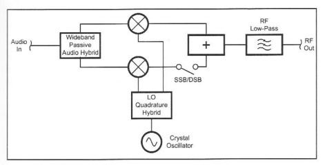
Fig 9.16-The exciter block diagram.
