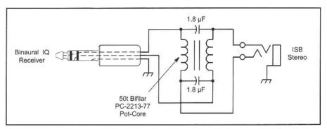
Fig 9.31-This outboard binaural network provides ISB headphone output.
