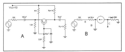
Fig 2.24—Common Base Amplifier with small-signal equivalent.
