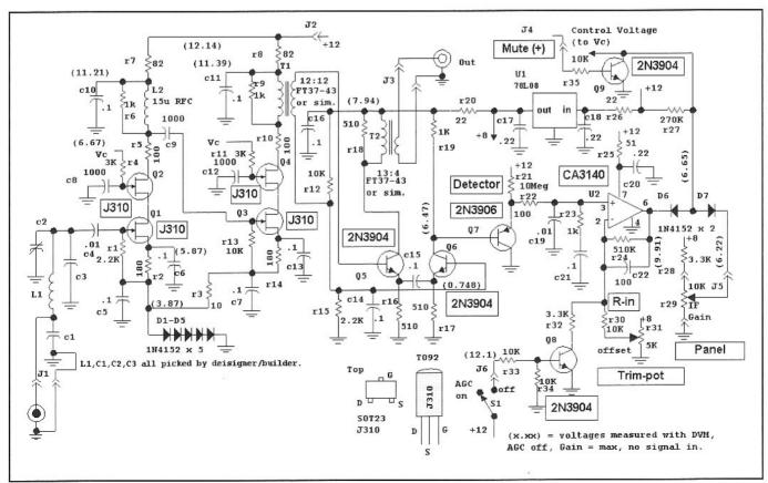
Fig 6.50—A general-purpose IF Amplifier module using cascode J310 JFETs. See text for details.
