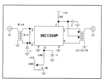
Fig 6.39—Amplifier for examination of the MC1350P. Gain is reduced by over 60 dB by increasing the dc current into pin 5.
