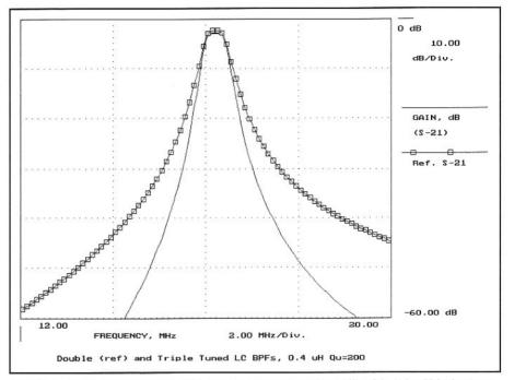
Fig 3.22—Response of triple and double-tuned circuits built with 0.4 mH inductors with  $Q_{\mu}$ =200.
