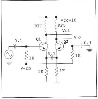
Fig 2.48—Differential Amplifier built with discrete components. The emitter resistors are adjusted for equal current in the two transistors.  $V_{bb}$  represents a base bias power supply, which could be a simple voltage divider from the higher supply.
