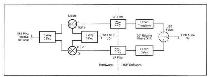
Fig 11.17—Simplified block diagram showing the phasing method of reception used in the 18-MHz transceiver. The circle at the right with a minus sign subtracts input signal 2 from input signal 1.
