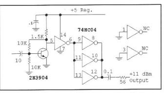
Fig 5.47—Simple limiting amplifier using a digital IC. Here, a HEX inverter generates an output with over 10 mW at the fundamental drive frequency. The inputs to unused sections should never be left floating.
