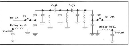
Fig 6.95—General form of preselector filters used for the high-performance receiver. While a 3-element filter is shown, some bands used up to 5 resonators.
