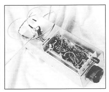
Fig 9.79—The interface circuit board connected between the R2pro ASP and a commercial IQ mixer operating at 2.3 GHz.
