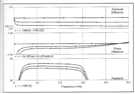
Fig 9.27—A *PSPICE* simulation result showing miniR2 diplexer amplitude and phase differences when the driving point impedance is 50, 75, and 100  $\Omega$ . This network is more tolerant of driving point impedance variations.
