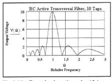
Fig 3.63—Transfer function of a 10-tap FIR filter.
