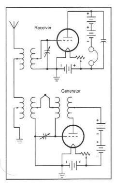
Fig 8.2—A classic radio enhanced with a local oscillator.
