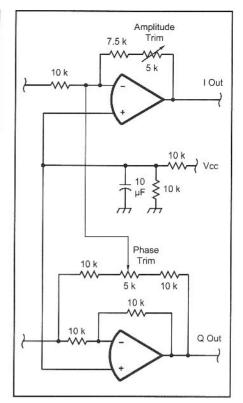
Fig 9.35—The op-amp circuit permits a small amount of Q-channel signal to be either added or subtracted to the I-channel signal.
