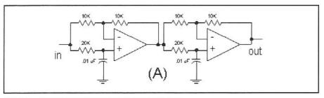
Fig 3.61—Half wave transmission line emulator.
