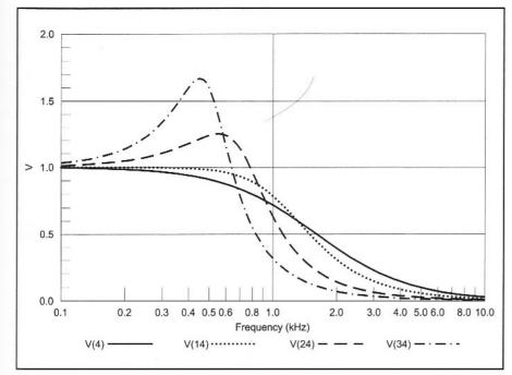
Fig 3.49—Response of the filter shown in Fig 3-48 with A=1, 2, 5, and 10. These curves, and several others in this section, were generated with *Super Spice* from Compact Software. The solid line corresponds to A=1 while the highest peak is for A=10.
