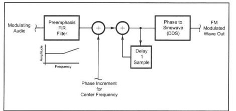
Fig 10.31—Direct generation of FM signal.
