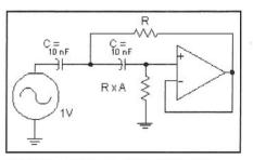
Fig 3.52—Voltage controlled voltage source high-pass filter. The operational amplifier is again set for a closed loop gain of +1.
