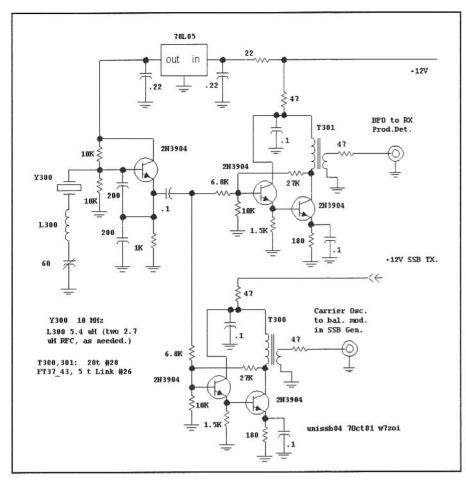
Fig 6.151—BFO and carrier generator. T301 and T300 each have a 15-turn primary with a 5-turn secondary on FT-37-43 cores. The amplifier input resistors, now 6.8  $k\Omega$ , can be changed to set the output power.
