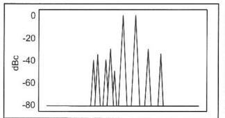
Fig 9.14—The spectrum of a typical SSB transmitter with twotone modulation, with the carrier suppressed 50 dB, 40 dB opposite sideband suppression, and amplifier intermod products 30 dB (3rd) and 35 dB (5th) below either of the two desired output frequencies.
