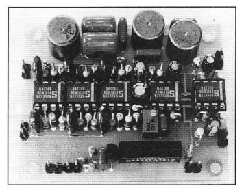
Fig 9.71—The analog signal processor.
