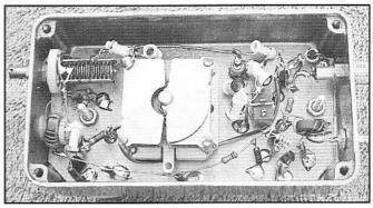
A clean way to fabricate an LC oscillator uses a Hammond 1590B box, offering excellent shielding. DC enters through a feedthrough capacitor and RF leaves on coaxial cable. This oscillator used a differential capacitor, but only one side is connected.
