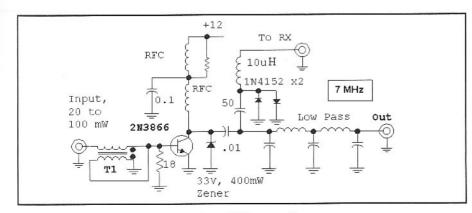
Fig 2.95-Typical output amplifier in a QRP transmitter.
