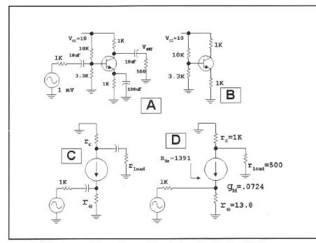
Fig 2.21—Single transistor audio amplifier design. See text for details.
