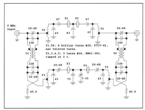
Fig 6.93—Crystal filter serving a "roofing" function. This circuit operates at 9 MHz, but can be redesigned for other frequencies within the HF spectrum. The variable capacitors with Y3 and Y4 are adjusted to match the one filter to the one using Y1 and Y2. The quadrature hybrids are adjusted for optimum impedance match at both ports. See text.
