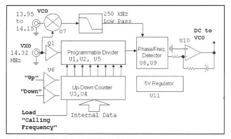
Fig 4.56—Block diagram for the VXO extending synthesizer.
