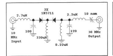
Fig 5.45—A simplified tripler circuit using only two diodes. This circuit is described in the Web site from Wenzel Associates. See text.
