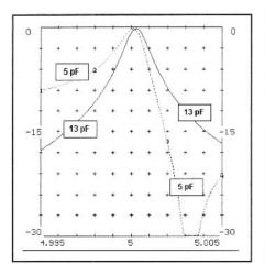
Fig 3.32—Response of the single crystal filter of Fig 3.31 when the phasing capacitor is at minimum value of 5 pF. The solid line represents the case of exact balance when the phasing capacitor equals the crystal  $C_0$ .
