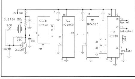
Fig 4.54—Time base portion of frequency counter.
