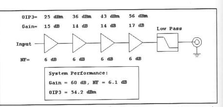
Fig 6.97—Individual stage parameters are combined for a cascade of four stages in an amplifier.
