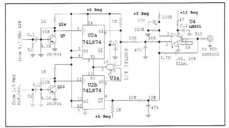
Fig 4.45—Phase-frequency detector and loop filter for the tracking PLL.
