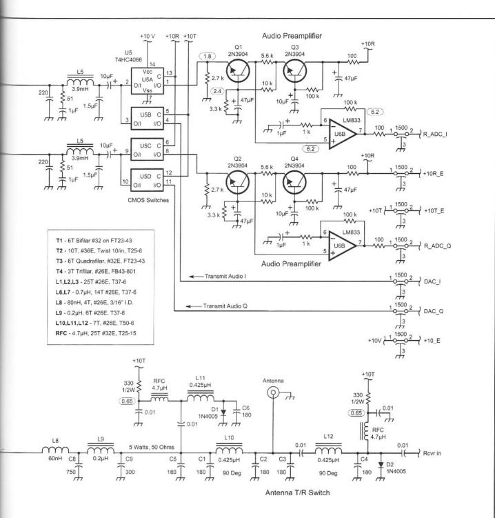
Note: The circuitry on these two pages (11.14 and 11.15) should be contained in a shielded enclosure. The 1500 pf feedthrough capacitors filter the leads coming into the enclosure.
