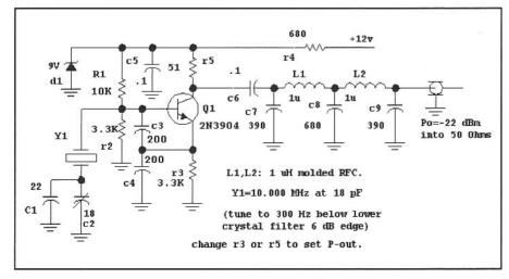
Fig 6.138—Carrier oscillator.
