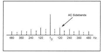
Fig 8.15-The spectrum of a re-radiated LO.
