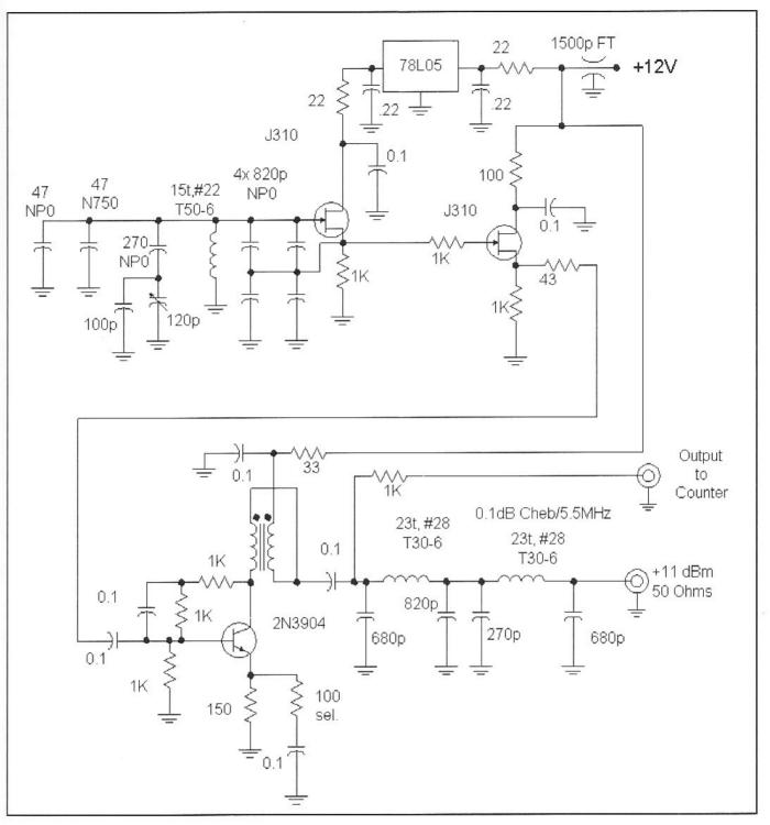
Fig 6.77—LO system for the 14-MHz receiver. The N750 capacitor provides temperature compensation as measured with a small homebuilt thermal chamber. All other capacitors in the oscillator have an NP0 temperature coefficient.
