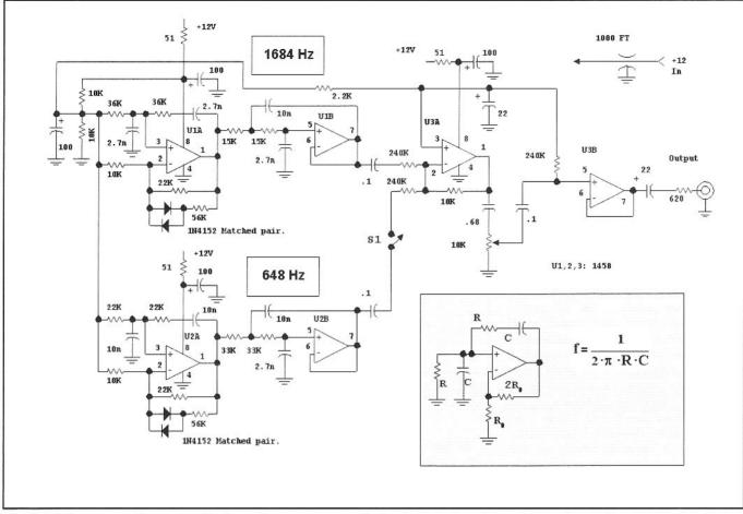
Fig 7.26—Two tone audio source. Each oscillator uses a matched pair of diodes with matching done with a DVM in the diode test position. Matching was done to 10 mV.
