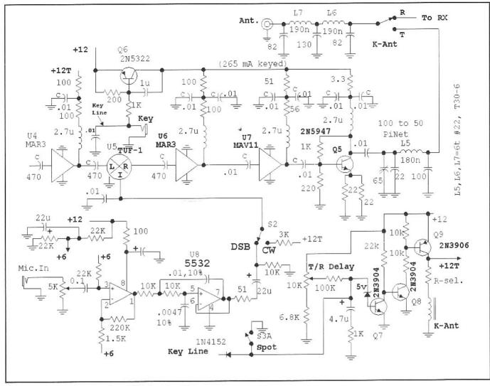
Fig 6.159-Transmitter portion of the 6-meter station.
