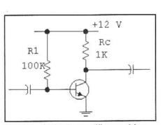
Fig 2.11—A simple amplifier used for bias analysis.
