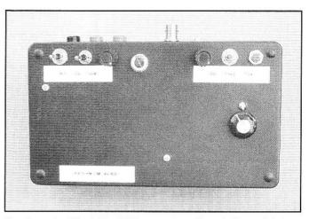
Front panel of Portable CW transceiver. The station weight, including batteries, earphones, keyer paddle, transmatch, and an end fed antenna, is about 2 pounds. The transceiver includes a bridge and VSWR indicating meter, so the transmatch consists of nothing more than the matching network.
