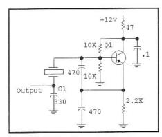
Fig 4.24—Method for extracting low noise, low distortion output from a crystal oscillator.
