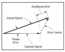
Fig 11.21—Phase and amplitude errors in the phasing method shown as vectors.
