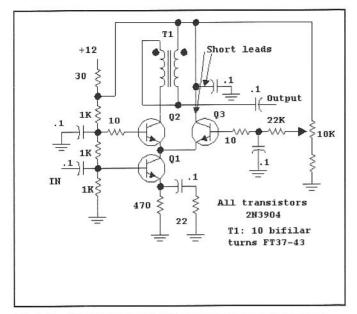
Fig 6.40—Bipolar transistor discrete IF amplifier with gain reduction using the same mechanism as used in the MC1350P. Control range was 70 dB, experimentally controlled with a 10-k $\Omega$  manual IF gain.
