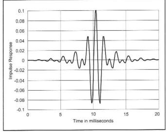
Fig 10.25—Impulse response of a Kaiser-window FIR filter designed for a center frequency of 800 Hz, using 200 coefficients and a sampling rate of 9600 Hz. The –6 dB-bandwidth was designed to be 500 Hz.
