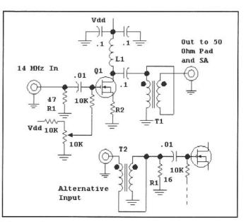
Fig 6.99—Class-A power amplifier experiment. Several MOSFET types were tried at Q1 while seeking high output intercept. L1 is 4  $\mu$ H of #22 wound on a T68-2 toroid. T1 is 10 bifilar turns #18 on an FT-82-43 ferrite toroid. T2 is 8 bifilar turns #22 on an FT-37-43. R1 should have a 1-W power rating. Class-A amplifiers like this should be mounted on a large heat sink, for efficiency is not a feature of the design. See text for details.
