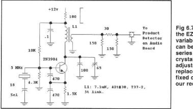
Fig 6.73—BFO for the EZ90-14C. A variable capacitor can be used in series with the crystal for final adjustment. It was replaced with a fixed capacitor in our receiver.
