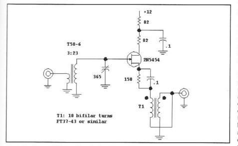
Fig 6.34—Source follower functioning as a low-noise amplifier. The drain resistor serves to suppress UHF parasitic oscillations. The components shown will tune from 6 to 22 MHz.
