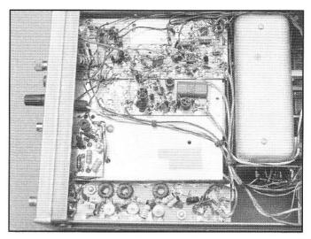
The bottom inside view of the "Unfinished-7" Transceiver. The upper circuitry includes audio, regulators, and sidetone. The board along the lower edge is the transmit mixer and triple tuned bandpass filter. The transmitter driver is the small board above the bandpass. The VFO module is at the right.
