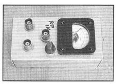
RF impedance bridge with built in meter. A reference must be attached for measurements.
