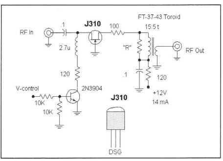
Fig 6.32—A common-gate amplifier using a JFET. The 100- $\Omega$  resistor at the drain suppresses UHF oscillations. See text regarding the drain load resistor, "R."
