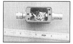
Interior view of return loss bridge. This one is built with 49.9  $\Omega$ , 0.1 W, 1% resistors.
