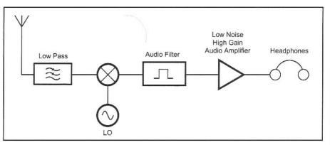
Fig 8.3—A block diagram of a basic direct-conversion receiver.
