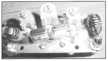
A close up photo of a 4th order filter built by WB4RNO. Any small trimmer capacitor with a suitably low minimum capacitance can be used.
