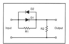
Fig 10.47—Schematic diagram of a simple gain expanding predistorter. This analog circuit is constrained by available diode types, but does provide a general gain characteristic that is opposite to that of amplifier gain compression.
