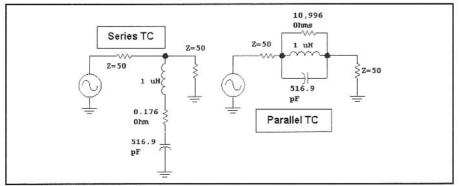
Fig 7.66—Measuring Q by determining the attenuation of a trap. A 7-MHz tuned circuit is used in this example with L=1  $\mu$ H. The 0.176- $\Omega$  resistor in the series-tuned circuit and the almost 11-k $\Omega$  resistor in the parallel tuned circuit are models representing a 7-MHz Q of 250. The series-tuned circuit (STC) will have an attenuation of 43.1 dB while the PTC has 40.9 dB.
