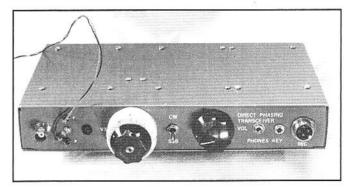
Fig 12.51-The Metal Box 144-MHz transceiver.
