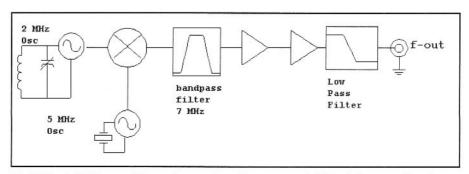
Fig 6.19—A CW transmitter using a mixer. Frequency stability is improved owing to use of a lower frequency for the variable-frequency oscillator. Careful bandpass filtering is required at the mixer output to preserve spectral purity.
