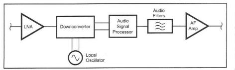
Fig 9.63—The R2pro block diagram.
