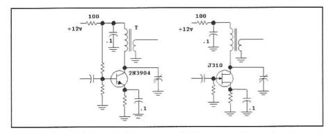
Fig 5.39—Simple, single-ended frequency multipliers using a bipolar transistor and a JFET. These classic circuits can still be useful in modern designs, but only if built with careful measurements.
