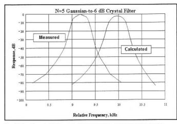
Fig 7.61—Crystal filter response for the circuit used in the measurement receiver. See text.
