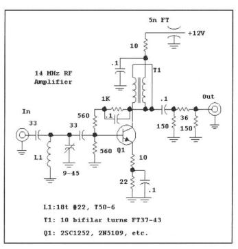
Fig 6.83—RF amplifier with preselector network. This amplifier used parallel feedback from the output tap. Feedback directly from the collector is preferred.
