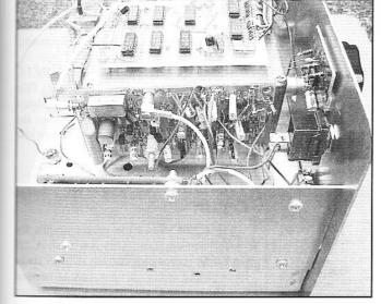
The audio amplifier and product detector board for the Universal Monoband Transceiver.
