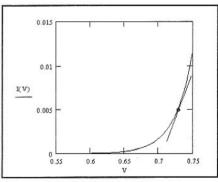
Fig 2.5—Small signal model for a junction diode represents it as a resistor with the slope shown. See text.
