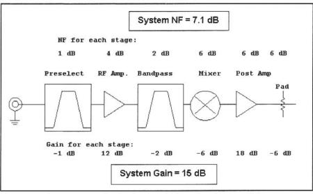
Fig 6.31—A six-stage cascade showing a typical receiver front end. The stages consist of a wide filter, an RF amplifier, a steeper skirted bandpass filter, a diode ring mixer, a post-mixer amplifier, and finally, a 6-dB attenuator.
