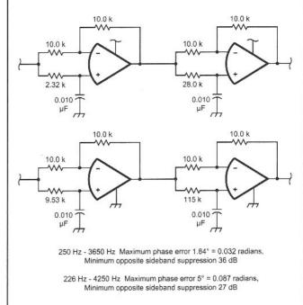
Fig 9.54—This second-order all-pass network provides more than 36 dB of opposite sideband suppression from 250 Hz to 3650 Hz for SSB operation.
