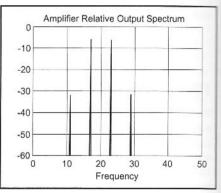
Fig 10.49—Amplifier output spectrum showing the two desired signals at frequencies of 17 and 23 and the thirdorder intermodulation products at frequencies of 12 and 29. These frequencies were chosen to be easy to simulate, but the results apply generally to any two-tone test frequencies. There are no intermodulation products of order higher than three, for the amplifier as it was modeled.
