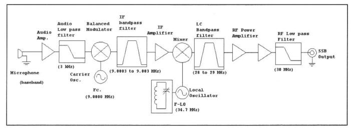
Fig 6.26—A practical filter type SSB transmitter where a mixer translates the output of a fixed-frequency SSB generator to a variety of outputs.
