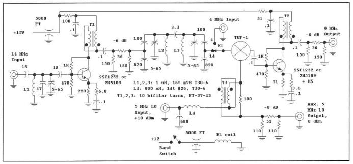
Fig 6.75—Front end for the 14-MHz receiver. The circuit is built largely with breadboarding methods.
