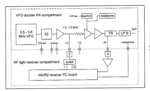
Fig 12.71—Block diagram of the Sleeping Bag Radio.
