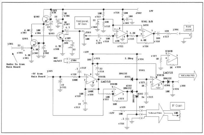
Fig 6.139—Audio system and AGC detector.
