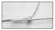
The end of a portable antenna requires no insulator. A tie-off cord or rope with the insulation on the wire is sufficient.
