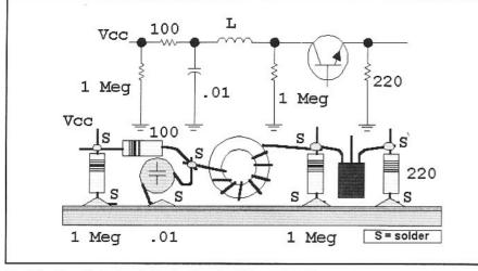
Fig 1.1—A partial circuit illustrating "ugly" construction.
