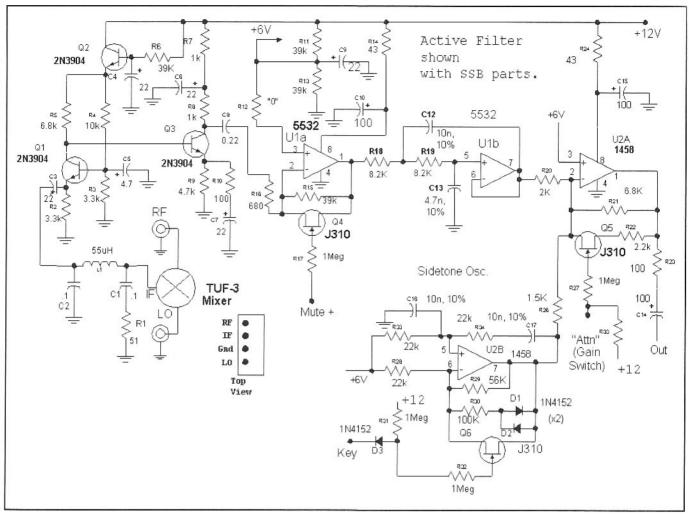
Fig 12.40—General-purpose direct-conversion receiver.
