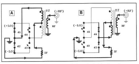
Fig 5.20—Diode ring commutating balanced mixers. See text for discussion.
