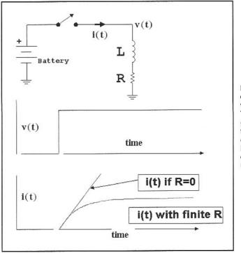
Fig 3.72—Principles of an ideal inductor, with waveforms. The current would grow linearly forever in an ideal component. Resistance establishes an ultimate value.
