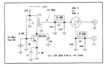
Fig 7.78— Receiving converter for experiments.
