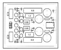
Fig 9.67—The downconverter board layout.
