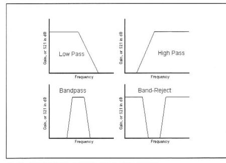
Fig 3.2—The frequency responses of various filter forms.
