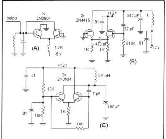
Fig 4.13—Negative resistance one-port oscillators for application at HF and VHF. See text for discussion.
