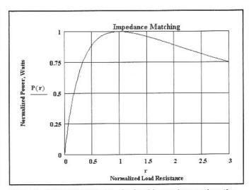
Fig 2.40—Power delivered to the load is maximum when the load resistance equals that of the source.
