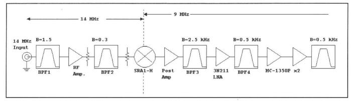
Fig 6.82—Block diagram of an early high-dynamic-range receiver. The various elements are shown in schematics. See text for stage-by-stage discussion.
