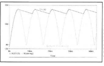
Fig 1.21— Waveforms for a simple power supply. The "before filtering" shows the raw rectified signal without any filter capacitor. The "Vcap" shows the voltage across the filter capacitor attached to the rectifier when loaded to a modest current.
