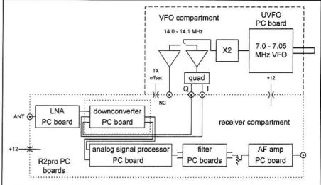
Fig 12.77—The 14-MHz R2pro block diagram.
