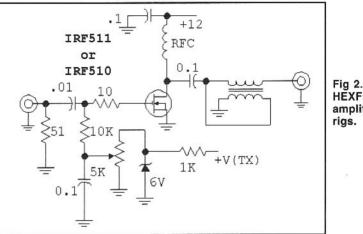
Fig 2.98—Simple HEXFET linear amplifier for QRP rigs.
