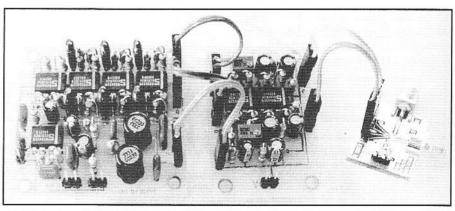
Fig 9.81—A prototype microwave SSB exciter connected to a commercial passive IQ FET mixer at 2.3 GHz.
