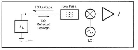
Fig 8.9—Local oscillator radiation.
