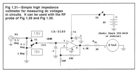
sured without upsetting signals that may be present in the circuit. This circuit can be calibrated with a fresh 1.5-V battery; vary the 6.2-k $\Omega$  resistor if needed.
