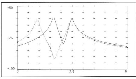
Fig 3.20—Separation of response peaks indicating coupling between two resonators. The solid line uses a 10-pF coupling capacitor while the dotted line uses 20 pF.
