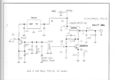
Fig 6.161—Eight megahertz VFO for the 6-m station receiver. Tank capacitors are selected to establish resonance at the desired operating frequency
