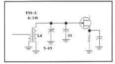
Fig 12.22—Single tuned mixer input circuit.
