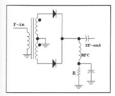
Fig 5.43—Improved balanced diode frequency doubler. Typical resistor values are from 10 to 220  $\Omega$ . See text.
