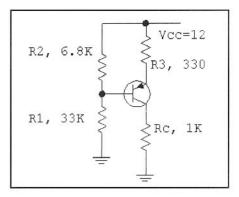
Fig 2.14—PNP biased to the same conditions as we established with the NPN example.
