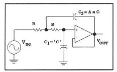
Fig 3.48—RC active low-pass filter. The op-amp is assumed to be powered from dual supplies around ground. Other biasing schemes are presented later. The operational amplifier is configured for a non-inverting gain of 1. C2, the feedback capacitor, is A x C1 where A is a value greater than 1.
