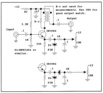
Fig 6.41—Simple gain-controlled amplifier. The inset shows the use of two PIN diodes to increase the control range slightly with the same control current. Many diode types work with this circuit; see text. The 10-k $\Omega$  pot establishes manual IF gain.
