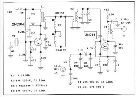
Fig 5.31—Schematic for a low noise 10.1-MHz converter.
