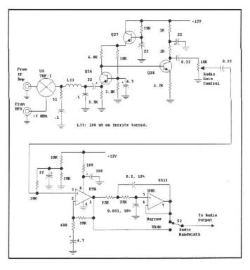
Fig 12.29— Product detector and audio amplifier. The emitter of Q28 may be bypassed for gain higher than needed here.
