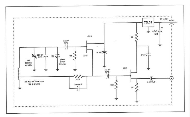
Fig 12.56-The 4.4-4.9 MHz VFO schematic
