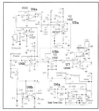
Fig 12.19—Audio output system. An RC active low pass filter, sidetone oscillator, 6-V regulator and T/R control are included.
