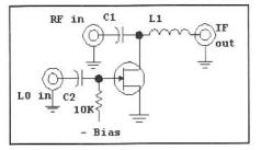
Fig 5.10—Switching mode mixer using a single FET. Although a JFET is shown, the mixer can also be implemented with a bipolar transistor, a MOSFET, or a GaAs FET. This circuit typically has a conversion loss of 6 dB. Input intercept (third order) can be from 0 to +20 dBm, depending on the FET type. LO energy at the RF port is typically reduced by 10 to 15 dB. Operating frequency will dictate the components in the diplexer filter, C1 and L1. See text.
