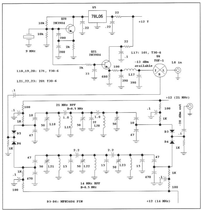
Fig 12.31—Transmit mixer with PIN diode switched bandpass filters. See text for details.
