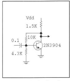
Fig 4.41—An analog signal is easily converted to digital form with the circuit shown here. The  $10-k\Omega$  and 4.3 $k\Omega$  resistors form a voltage divider with a voltage gain of about 1/3. But, to be active, the transistor base must be biased at about 0.7 V.
