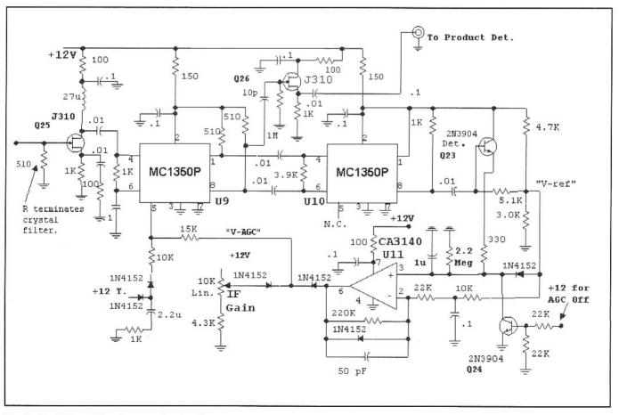
Fig 12.15—IF Amplifier. See text for details.
