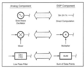
Fig 10.37—Equivalent analog and DSP components that are used to create an "equivelent circuit" for the discrete Fourier transform (DFT).
