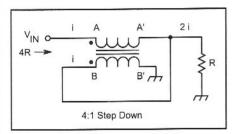
Fig 3.77—A single ended impedance step down transformer.
