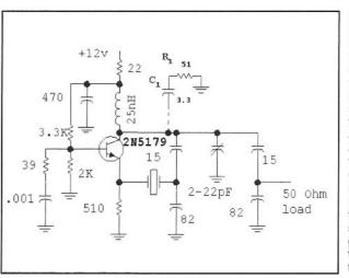
Fig 4.28-Butler oscillator for 100 MHz. L=25 nH. This is formed with a 1.7 inch piece of #22 enameled wire wound in the threads of a 6-32 machine screw.(3.3 mm dia, 12.6 turns/cm) The wire ends are stripped and 3 turns are wound on the screw, which is then removed. C1 and R1 form a network to suppress UHF oscillations at 500 to 1000 MHz. The suppression circuit generates a UHF load that is largely absent at the operating frequency.
