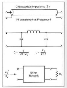
Fig 11.15—Schematics and design equations for impedance inverters built from transmission lines and lumped capacitors and inductors. At the single frequency, f, the two circuits have identical behavior.
