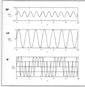
Fig 5.21—Waveforms for a diode ring commutation mixer. The RF and LO signals are those seen when the sources are examined into resistive loads. The IF signal is merely the RF waveform, except that the polarity is reversed when the LO is negative.
