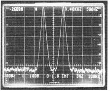
Fig 10.5—D/A output spectrum for two sine waves at 8.9 and 9.9 kHz. Each signal was 2.0 V p-p so that the peak level for both sine waves was 4.0 V p-p, which is full scale for the D/A converter. The noise floor, which is about 65 dB below each of the sine waves, is mainly from the spectrum analyzer.
