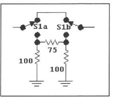
Fig 6.36—A 50- $\Omega$ , 10-dB pad using standard resistors and a toggle switch. Short lead lengths should be used to provide good performance over the HF region. Relay switching could also be used.
