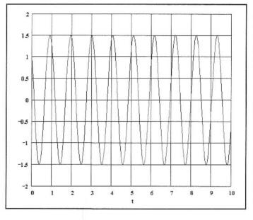
Fig 7.5-The appearance of an oscilloscope faceplate while examining a sinusoid. This ac voltage moves from zero to 1.5 V, back to zero, to -1.5, and again to zero, with the sequence repeating for a long time. This signal is measured as 3 V peak-to-peak. The display shown has a vertical sensitivity setting of 0.5 V per division.
