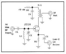
Fig 5.6—JFET mixer with a wideband output termination using a 5:1 turns ratio transformer. LO power is applied to the source, but this still results in LO between the source and drain, making this circuit the equivalent of Fig 5.2.
