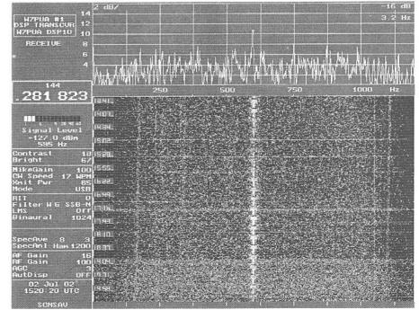
Fig 10.41—A Spectrum Analyzer display while receiving weak signals with the DSP-10. Signals below about –150 dBm are too weak to be heard by the ear, but the narrow bandwidths of the DFT make these easily seen on the display.
