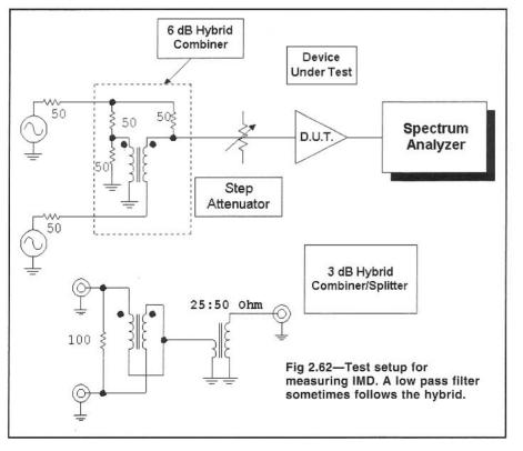
$(f_1+f_2)$  and  $(f_1-f_2)$ . These distortion frequencies are usually far removed from the inputs. Hence, they can be removed with a filter following the amplifier. This is not possible with third order products very close to the frequencies causing the distortion.
