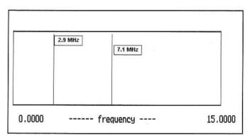
Fig 5.13—Idealized mixer output for the circuit of Fig 5.12 without the output filter.
