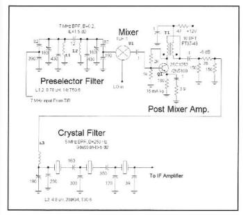
Fig 12.14—Receiver front end for the Unfinished. A Gaussianto-6 dB shaped crystal filter is included. The double-tuned circuit is not symmetric, because an adjustment was made to compensate for interaction with the tuned circuit in the T/R system.
