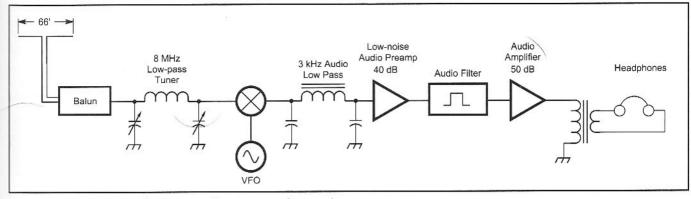
Fig 8.4—Block diagram of a 40-meter direct-conversion receiver.
