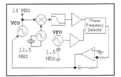
Fig 4.42—A practical one-on-one or offset tracking PLL.
