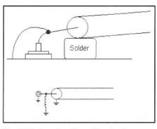
Fig 3.26—Loading (coupling to the "outside world") can be controlled with small wire inductors.
