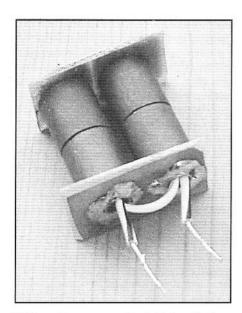
RF transformers can be built by placing ferrite beads over brass tubing that forms a single turn winding. Circuit board material connects the tubing ends with a short at one end. A multiple wire winding is then threaded through the middle of the tubing, guaranteeing tight coupling.
