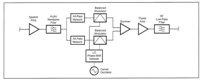
Fig 9.2-Block diagram of a phasing SSB exciter.
