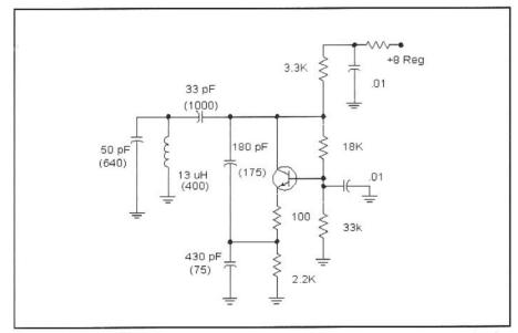
Fig 4.11—A Seiler oscillator for 5-MHz operation. The values shown in parenthesis are reactances, allowing the circuit to be scaled to other frequencies. Transistor type is not critical, although the circuit works well with a 2N3904.
