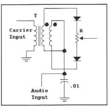
Fig 6.100—Simple balanced modulator for use in simple transmitters. R can be a small trim pot with R from 100  $\Omega$ to 2 k $\Omega$ . T is 10 bifilar turns on an FT-37-43 for HF applications.
