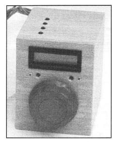
The knob box was built from thin plywood. An inner box made from scrap circuit board material contains the logic circuitry shown in Fig 11.7. The four push buttons are placed on the top of the box as a convenience in using the box. It is light enough that it wants to move when the buttons are pushed! The LCD display is above the knob. A plastic bezel trims off the display.
