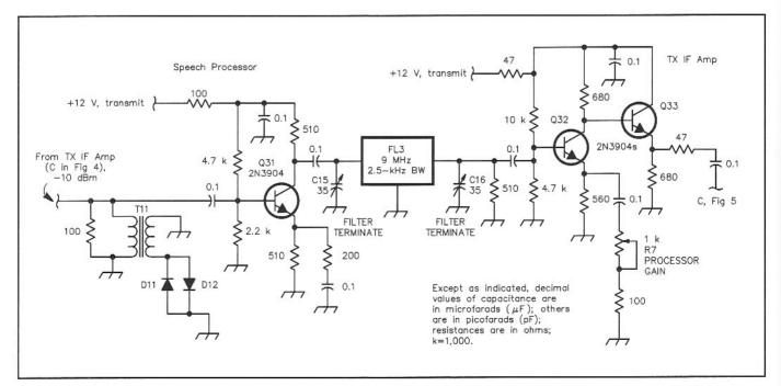
Fig 6.107—IF speech processor. Back-to-back diodes clip the IF signal. The resulting voltage is amplified and filtered in a crystal filter. It is then amplified and set to provide the desired –10 dBm to drive the transmit mixer. Schottky diodes are used in the clipper circuit. The diodes are driven by a 16-turn winding on an FT-37-43 ferrite toroid. The link on the  $50-\Omega$  line is 3 turns.
