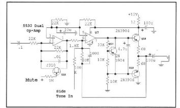
Fig 12.30—An audio output amplifier for the receiver.
