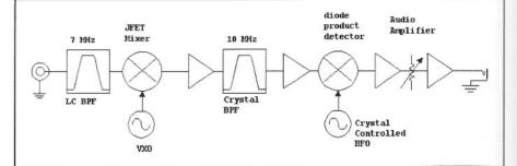
Fig 12.20-Block diagram for the S7C.
