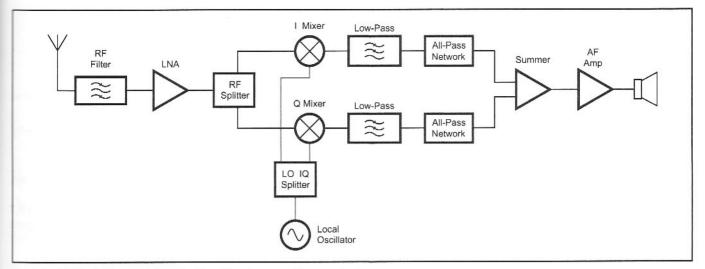
Fig 9.5—A block diagram of a phasing direct conversion receiver.
