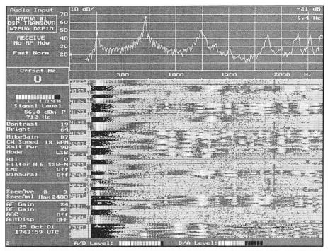
Fig 11.34—Audio processor display with operation on 10-meter CW. The top graph is the latest measured audio spectrum, which is updated every 0.6 seconds. Each of the approximately ten peaks are CW stations. The lower waterfall display shows the signal strength for each frequency plotted downward as time progresses. The time in minutes and seconds is shown at the left edge of the waterfall display. As explained in the text, brighter colors on the waterfall represent stronger signals.
