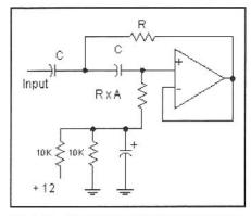
Fig 3.54—Biasing method for high-pass filter sections. A voltage divider creates a synthetic ground at half of the single supply.
