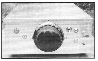
Front panel view. Switch between tuning and audio gain is a sub-band switch. The pushbutton injects an audio tone for tuning.
