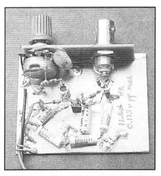
A simple audio oscillator for transmitter testing.
