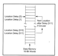
Fig 11.23—Circular data buffer used to implement a 512 point delay line as is used for delay binaural operation.
