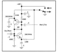
Fig 6.110—Bidirectional amplifier with complementary transistors. Only one transistor is on for each direction. Operation is clear if one of the transistors is mentally removed and the remaining circuitry is analyzed. See text for details.
