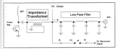
Fig 6.123—The RF portion of a T/R switch using a single switch. The transmitter is always connected to the antenna.
