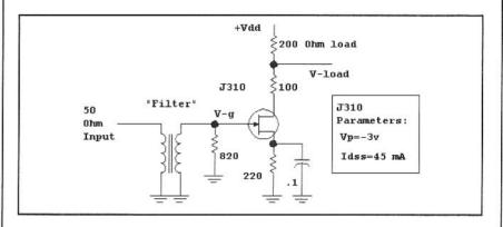
The "filter" is the combination of an impedance-transforming network and a crystal filter in this instance. The 50- $\Omega$  source is transformed to match a higher resistance, 820  $\Omega$  in the schematic above, with the composite "filter."
