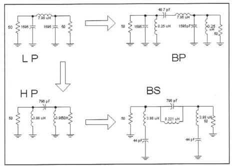
Fig 3.12—A low-pass filter (LP) is the prototype for the high pass (HP). The components in the low pass may be resonated to produce a bandpass (BP) filter with a bandwidth equaling the original low pass. Similarly, the high-pass elements are tuned to produce a bandstop filter (BS) with a 3-dB notch width equaling the bandwidth of the high pass.
