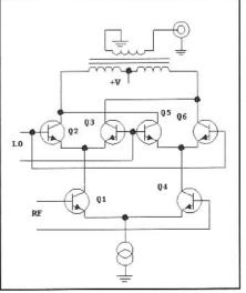
Fig 5.25—Fundamental Gilbert Cell mixer. The collector load is sometimes realized with resistors, although this will degrade intercepts, for internal load resistors absorb power that would otherwise be available to an external load.
