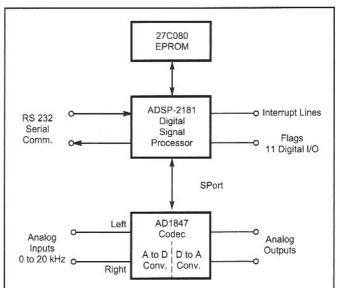
Fig 10.2—Block diagram of the EZ-Kit Lite from Analog Devices. The CODEC has dual A/D and D/A converters. Memory in the ADSP-2181 can be loaded from the EPROM. trol purposes and connections are supplied for adding almost any kind of memory or I/O device.
