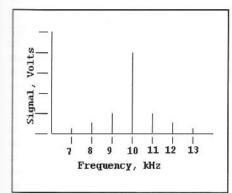
Fig 6.17—Spectrum of an FM signal, 10-kHz carrier with 1-kHz audio. This graph represents what we might observe with a typical spectrum analyzer. We often see plots like this with some components below the frequency axis, indicating a sign change when frequency is modulated rather than amplitude.
