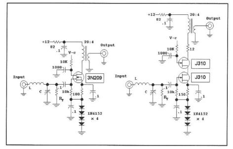
Fig 6.45—An IF amplifier using either a dual-gate MOSFET or a cascode connection of JFETs. These amplifiers use diode strings in series with the FETs for biasing, allowing substantial gain reduction with reduced control voltage. Transformers use #28 wire on an FT-37-43 ferrite toroid. Measurements were done at 10 or 14 MHz.
