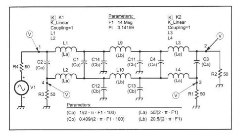
Fig 9.39—The LO quadrature network has wideband phase balance and acceptable amplitude balance over any amateur band, and the combined lowpass filter-splitter for RF provides a natural and well-behaved phase adjustment point. Here we move the phase adjustment to the LO path.
