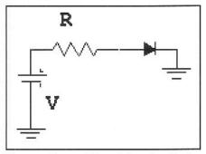
Fig 2.1—Forward biased junction diode.
