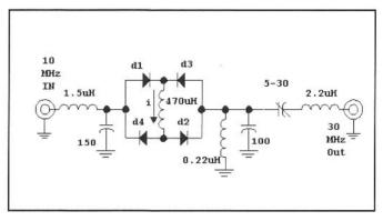
Fig 5.44— Frequency tripler using four diodes and a large inductance choke to generate a square wave. The output circuits are tuned to the 3rd harmonic of the input drive.
