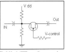
Fig 2.26—A JFET operating as a series switch.
