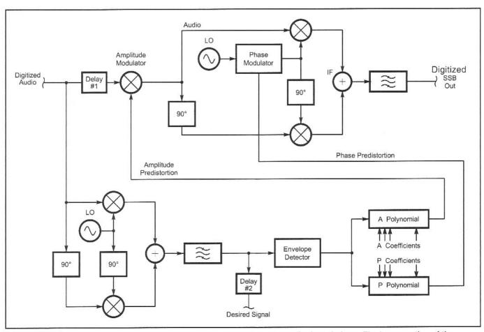
Fig 10.53—Block diagram of a SSB transmitter with predistortion in both amplitude and phase. The lower portion of the diagram is conventional phasing type of SSB generator that serves to determine the desired envelope amplitude, which determines the polynomial predistortion. All components shown are implemented in DSP.
