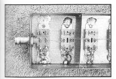
A step attenuator for the HF spectrum is easily built with slide switches and 1/4-W resistors. This design used a brass box with the switches soldered in place. This was hard on the plastic parts of the switches, making hardware mounting preferred.
