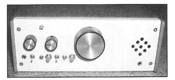
Front panel of 75-meter version built by AA7QU. One of the buttons activates a "Freq-Mite" frequency keyer that then reads the frequency and presents it in morse code.
