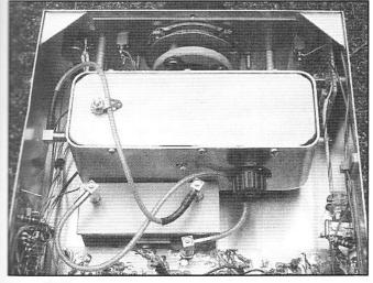
RF Power chain. The HEX-FET PA is normally attached to the cabinet that serves as a heat sink.
