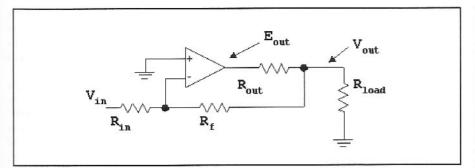
Fig 2.54—Feedback reduces an output resistance.
