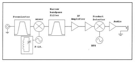
Fig 6.27—A traditional superhet SSB receiver. The response from only one sideband is allowed owing to the narrow-bandwidth crystal filter and the relationship of the BFO frequency to that filter.
