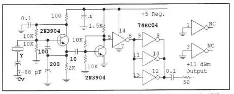
Fig 4.31—Adding HCMOS inverters can substantially flatten the output of a VXO. Output filtering will be required.
