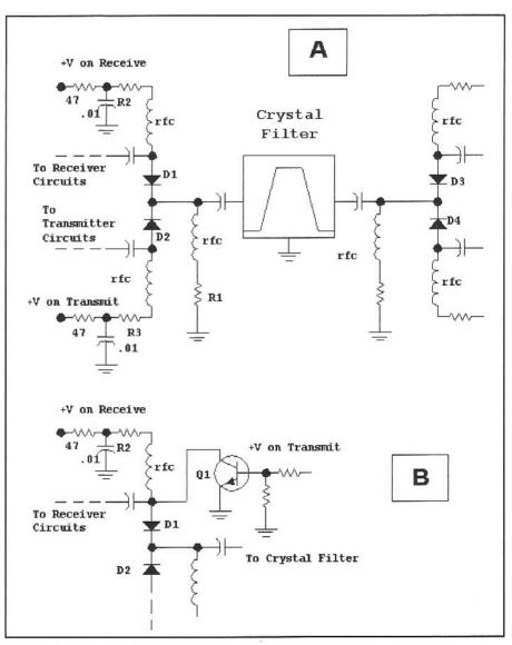
Fig 6.112—Diode switching of a crystal filter between transmit and receive functions. See text for details.
