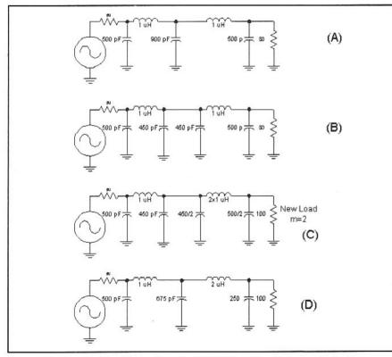
Fig 3.9—Low-pass filter illustrating Bartlett's Bisection Theorem that allows a termination to be changed to a new value.
