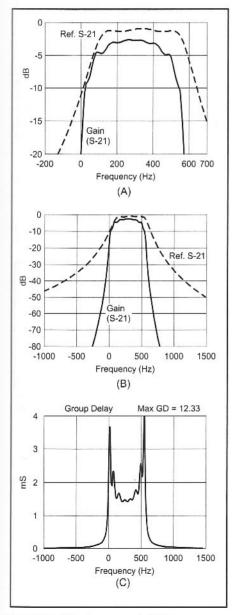
Fig 3.44—Min-Loss crystal filter responses. A and B compare 3rd and 8th order filters in responses to -20 and -80 dB. C shows the group delay for the 8th order filter.
