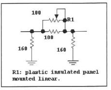
Fig 7.22—Continuously variable attenuator with about a 4-dB range.
