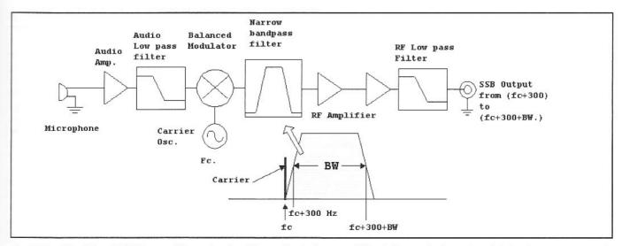
Fig 6.25—A traditional SSB transmitter using the filter method. A narrow filter follows a balanced modulator to remove one of two sidebands present on the DSB output of the modulator.
