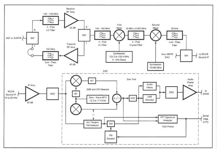
Fig 11.31—Overall block diagram for the DSP-10 2-meter transceiver. The portion inside the dashed lines is implemented as a DSP program. Not shown here are the control and display functions that are implemented in a PC.
