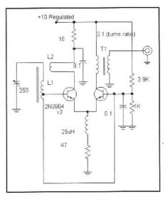
Fig 4.18—Low Noise 10-MHz Oscillator designed by K7HFD. L1 is 1.2  $\mu$ H, consisting of 17 turns on a T68-6 toroid core. The tap is at 1 turn from the grounded end while the link is 2 turns wound over L1. The link must be properly phased for oscillation. Although not shown, ferrite beads were used on both bases and collectors.
