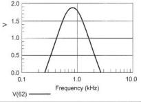
Fig 3.55—The 4x4 filter, a cascade of four peaked low-pass sections (6.8 k $\Omega$ , 10 nF, and 50 nF) followed by four peaked high-pass sections (20 nF, 27 k $\Omega$ , and 5.6 k $\Omega$ )
