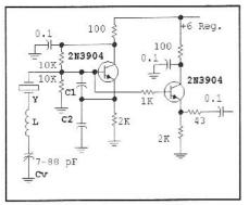
Fig 4.30—Basic VXO circuit. C2 is typically twice C1, which is 100 pF at 10 MHz and higher, doubling for 7 MHz. L is determined by experiment. C<sub>v</sub> can be about any variable capacitor, but should be one with small minimum capacitance. L may = 0, 2.7  $\mu$ H or 5.4  $\mu$ H.
