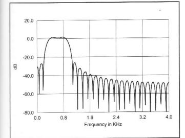
Fig 10.21—Response Curve for the 50-coefficient FIR filter of Fig 10.20 when using a 30-dB Kaiser windowing function to reduce the out-of-band response.
