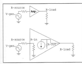
Fig 2.38—Basic amplifier with resistive input and output impedances.
