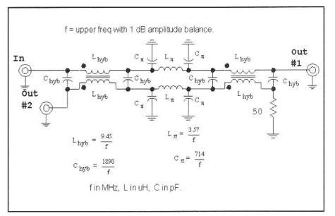
Fig 3.87—Extended bandwidth quadrature hybrid network.
