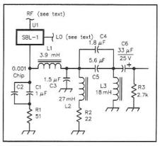
Fig 9.24—The complete schematic of the bandpass diplexer used in the R2.
