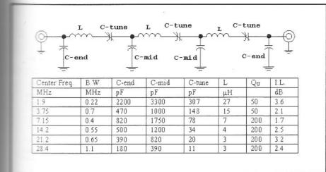
Fig 5.135—Triple-tuned bandpass filters for several HF bands. The required unloaded Q (vital) is also given.
