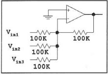
Fig 2.53—A summing amplifier with three inputs.
