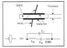
Fig 4.22—Cross-section, symbol and model for a quartz crystal.
