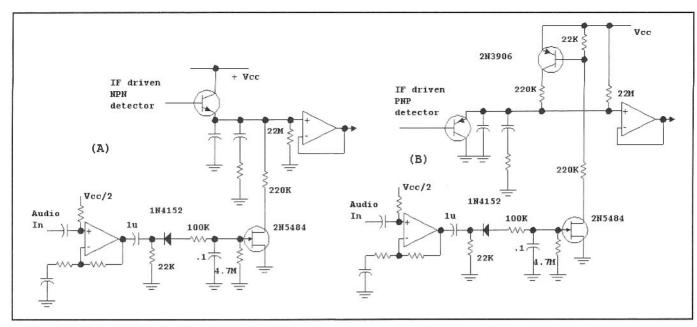
Fig 6.58—Adapting a hang AGC to IF amplifiers with NPN or PNP detectors. See text discussion.
