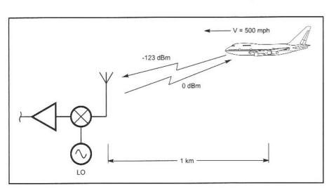
Fig 8.12—2-m radiation from an airplane 1 km away.
