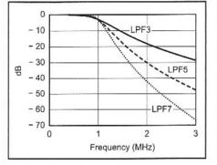
Fig 3.4—Transfer function for low-pass filters with order 3, 5 and 7. Adding sections will increase stopband attenuation.
