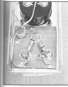
Symmetry and short lead lengths are maintained during construction. Long leads are okay with the dc parts of the circuit.
