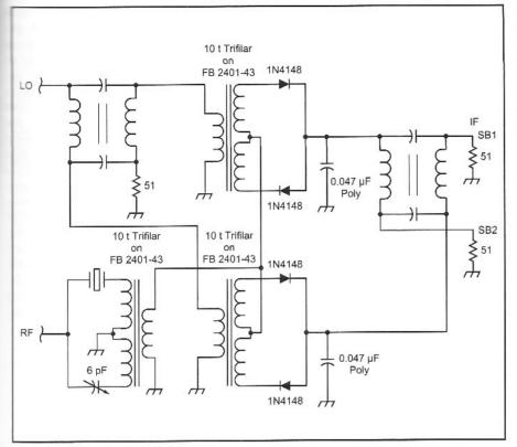
Fig 9.12—If the product detector is operated at a fixed frequency, crystal filter selectivity may be combined with a phasing product detector. This figure shows the basic circuit with a single-crystal CW filter connected directly to the product detector. It doesn't work as expected.
