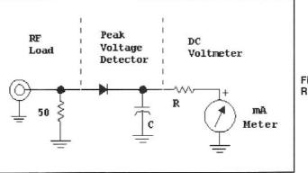
Fig 1.25—A basic RF power meter. the radio frequency applied to it. This means that the usual power resistors sold by vendors, even if capable of dissipating 100 W, will not be suitable. They are usually built as a "wire wound" part, making them highly inductive for RF. It is sometimes possible to tune them, an interesting avenue for the advanced experimenter.
