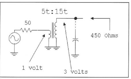
Fig 3.70—Circuit illustrating the transfer characteristics of an ideal transformer.
