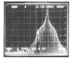
Fig 11.27—Measured spectrum of the transceiver in CW, when being keyed on and off at 10 dots/sec. The horizontal scale is 500 Hz/div and the vertical scale is 10 dB/div.
