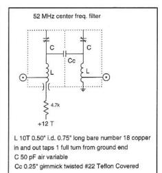
Fig 12.63-The 52-MHz filter.
