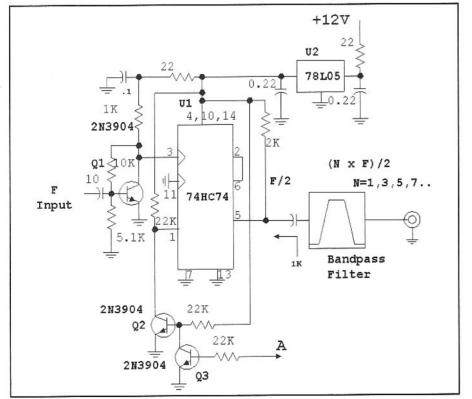
Fig 5.46—This frequency multiplier begins with a frequency division by 2 in a digital integrated circuit. The result, after division, is a very precise square wave. Odd harmonics can then be selected with a suitable bandpass filter. The output from the filter is typically –5 dBm when n=3. The bandpass should be designed for a termination of 1 k $\Omega$  at the IC end.
