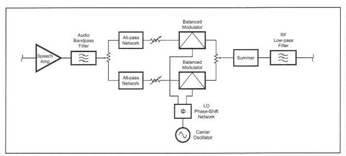
Fig 9.33—Possible locations for the amplitude balance adjustment in exciters.
