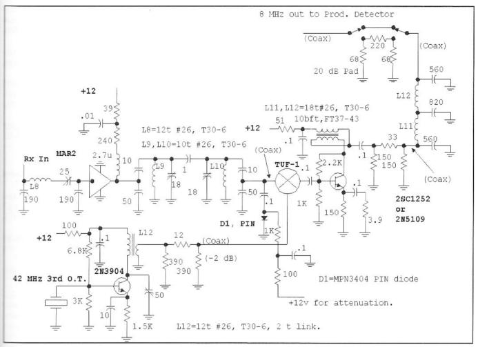
Fig 6.160-Receiving converter used with the 6-m portable station.
