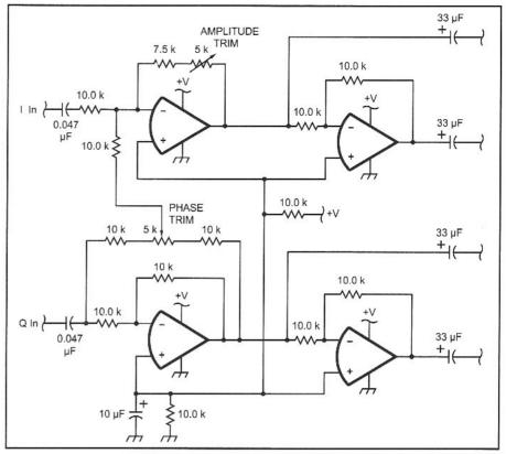
Fig 9.80—A circuit that provides dc-isolated balanced I and balanced Q drive to the inputs of an I Q upconverter.
