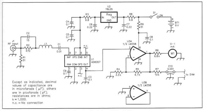
Fig 7.13-Logarithmic power meter capable of reading signals from -80 to +13 dBm.
