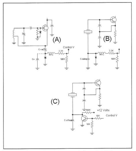
Fig 6.116—Oscillator circuits, including a means for frequency shifting.
