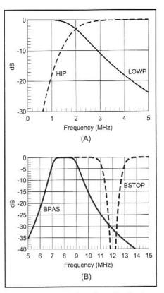
Fig 3.13—Transfer functions for the low pass and high pass (A) and the bandpass and bandstop filters (B).
