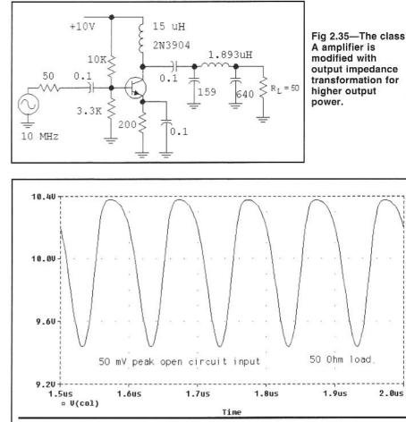
Fig 2.36—50- $\Omega$  termination on the class A amplifier.
