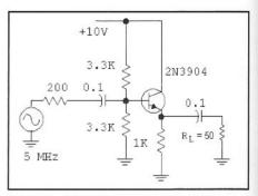
Fig 2.31—Emitter follower to drive a 50- $\Omega$  load. This circuit is not biased to deliver the needed output power.
