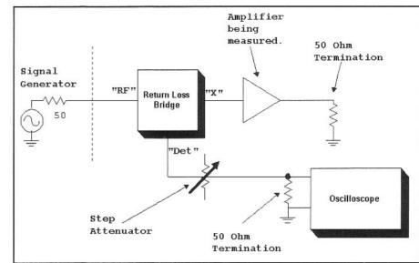
Fig 2.45—Using a return loss bridge with an amplifier.
