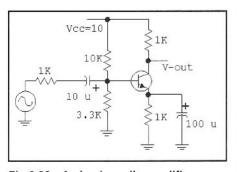
Fig 2.29—A simple audio amplifier examined for large signal performance.
