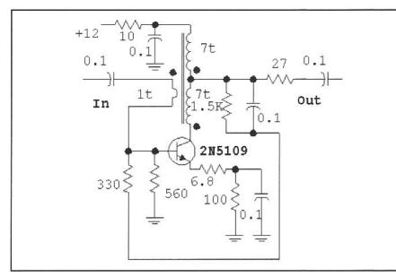
Fig 2.82—A modified feedback amplifier where transformer feedback increases input impedance.
