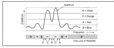
Fig 11.32—Diagram showing how the upper spectral is "sliced" into colors to form the one line of the waterfall display. While this simplified diagram has only four colors, the waterfalls usually have 16 colors or more. Added colors improve the ability to see weak signals against a noise background.
