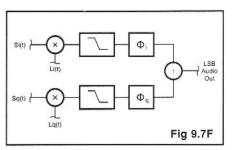
Note that the equal and opposite signal components have added to zero, and only the error terms remain. Also note that the effect of a 0.1-radian phase error is identical to the effect of a 0.1 amplitude error. Finally, note that the two error terms are orthogonal (one is a sine, and the other is a cosine), so that each must be independently reduced to zero—an amplitude error will not cancel a phase error. The two error voltages add to make a resultant error signal, with magnitude:
