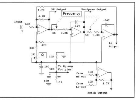
Fig 3.58—State-variable audio filter for CW receiver applications. All op-amps are 741 or 1458. The op-amp pin numbers are not shown. The builder must also connect the power supply line to the  $V_{cc}$  point on the op-amps. This circuit was inserted between the audio gain control and the output amplifier in a high performance CW receiver.
