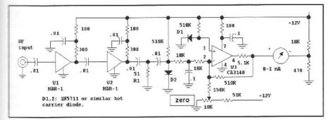
Fig 7.12—Low-level power meter capable of well under 1  $\mu$ W full scale. This circuit is calibrated against a calibrated signal generator, or against an attenuated QRP transmitter that has been measured with a simple power meter.
