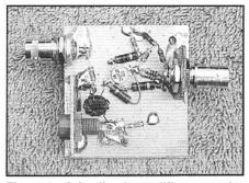
Fig 2.84—A feedback amplifier example. This circuit supplements test equipment. With  $V_{cc}$ =12,  $I_c$ =65 mA and OIP3=+42 dBm, Gain=16 dB, and bandwidth exceeds 50 MHz.
