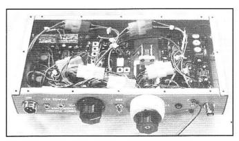
Fig 12.52—An inside look at the Metal Box 144-MHz transceiver.
