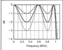
Fig 3.6—Chebyshev 5th-order low-pass filter transfer functions showing passband ripples of 1, 2, and 3 dB. These extreme ripple values are rarely used, but illustrate the concepts. Note that there is a half cycle of ripple for each filter element.
