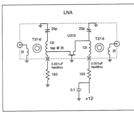
Fig 12.55—LNA schematic.
