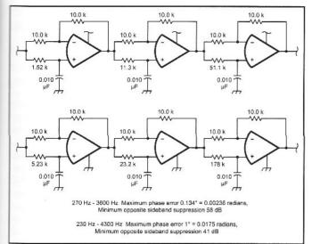
Fig 9.56—Adding a third pair of op-amps allows us to build a network with small enough amplitude and phase errors that we could achieve almost 60 dB of sideband suppression from 270 Hz through 3600 Hz, if the rest of the receiver were perfect.
