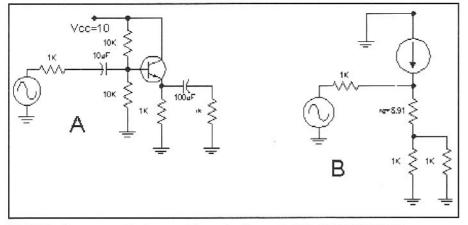
Fig 2.22—Common collector amplifier, also known as an emitter follower.
