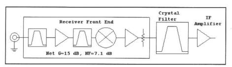
Fig 6.38—The front end presented earlier in Fig 6.31 is combined with a crystal filter of known insertion loss, followed by an IF amplifier. If the filter has a 10-dB IL, a 7-dB IF noise figure will produce a system NF of 10.6 dB.
