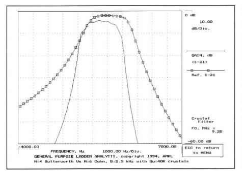
Fig 6.147—Crystal filter responses for two crystal filters. The Cohn is the preferred design for this transceiver even though the low crystal Q<sub>u</sub> rounds the passband corners. See text.
