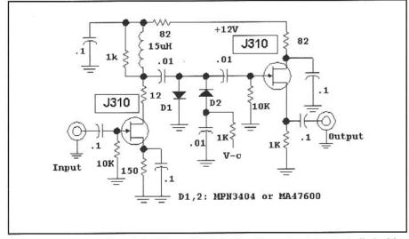
Fig 6.42—AGC amplifier with FETs and PIN diodes. Manual gain is controlled with the 10-k $\Omega$  pot.
