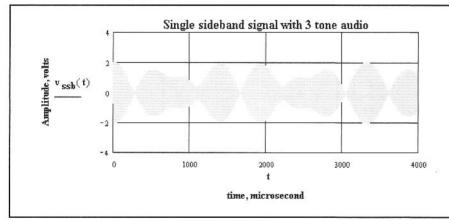
Fig 6.13-Single-sideband signal from a three-tone baseband input.
