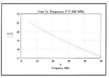
Fig 2.76—Feedback tends to flatten frequency response. This is even more dramatic with lower gain amplifiers.
