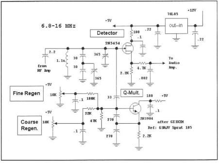
Fig 1.16—Alternative regenerative detector.
