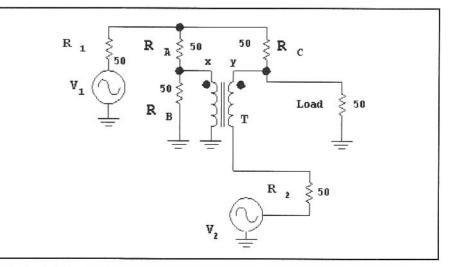
Fig 7.42—A RLB also finds use in combining two signal generators. The power delivered to the load is 1/4 of that available from each generator when the bridge is balanced.
