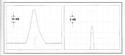
Fig 7.55—A 10 dB/div. signal at the left is adjusted to fill much of the screen. Switching to 2 dB/div. produces the display at the right. Adjusting the offset controls R1 and R2 allows moving the response anywhere on the CRT screen.
