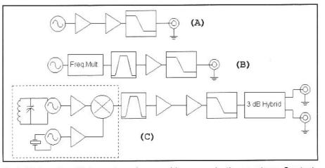
Fig 6.80—Local-oscillator systems for use with communications systems. See text for details.
