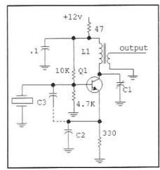
Fig 4.26—General purpose power oscillator for use from 2 to 70 MHz. Q1 is a 2N3904 or similar medium  $F_T$  device. See text for component value discussion.
