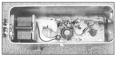
This Hartley Oscillator is mounted in a stamped box. A vernier drive is attached to the capacitor shaft and is fixed to the box with a single bolt that prevents rotation. Spade lugs allow a lid to be attached to the box.
