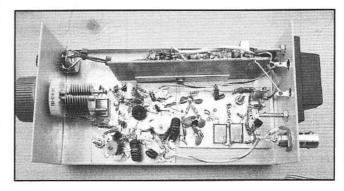
Top inside view of the simple superhet receiver. The left board houses the front-end mixer and the VXO. The board at the right contains the IF and crystal filter. The power connector uses a quick disconnect normally used with audio speaker cables.
