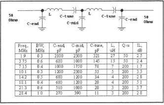
Fig 6.133—Receiver bandpass filters using series resonators.
