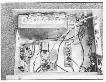
The audio amplifier and product detector for 8-MHz directconversion IF system are all in a Hammond 1590B box with coax and feedthrough capacitor interface connections. The 42-MHz crystal oscillator and 8-MHz low pass filter are on the small boards. The long board across the bottom of the figure is the VXO and ×3.5 frequency multiplier chain.
