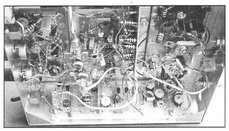
General-purpose receiver front end board installed in the EZ90-14 Receiver.
