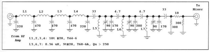
Fig 6.84—Image-stripping preselector filter used with the receiver. This filter provides over 100-dB suppression of images and other spurious responses.
