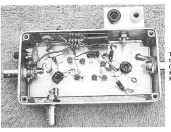
The Ditter for AGC testing in a receiver. (Thanks for circuit suggestion from K7RO)
