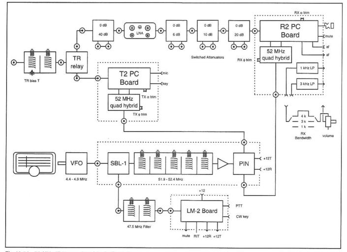
Fig 12.54—52-MHz IF transceiver block diagram.
