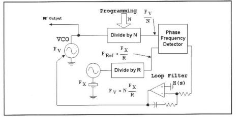
Fig 4.46—A single loop Divide-by-N PLL.
