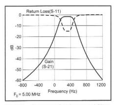
Fig 3.38—Response for the crystal filter designed in Fig 3.37.
