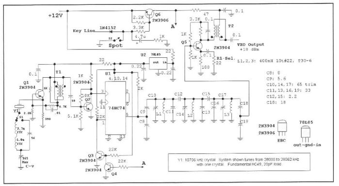
Fig 12.37—An 18.7-MHz VXO (Q1) is frequency divided by 2 with U1 to form a square wave. The third harmonic is selected with the bandpass filter and amplified to a 10-milliwatt output level. T1 is 10 bifilar turns #28 on an FT-37-43. S1 is a wafer switch with low capacitance. A toggle switch should *not* be used here.
