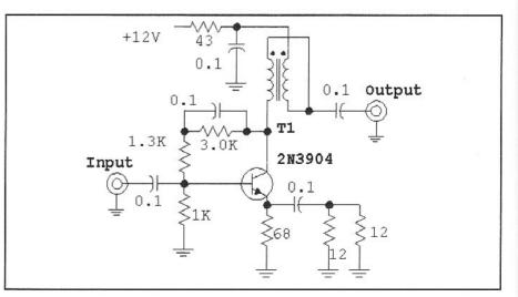
Fig 2.57—Feedback amplifier illustrating gain compression and distortion. This circuit has 20-mA I<sub>c</sub>. T<sub>1</sub> consists of 10 bifilar turns on a FT-37-43 ferrite toroid core, although the specific core type is not critical. This circuit features a small signal gain of 20.5 dB and a good impedance match to 50  $\Omega$  at both input and output. See text for noise Figure, gain compression, and intercept results.
