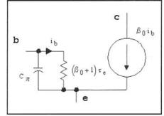
Fig 2.28—The hybrid-pi transistor model.
