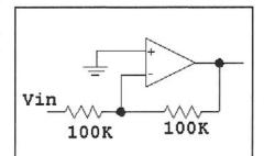
Fig 2.52—An inverting amplifier with unity gain.
