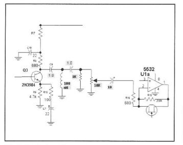
Fig 12.41—Option with an added audio gain control. Also shown is an LC high pass filter. The altered or added components are highlighted.
