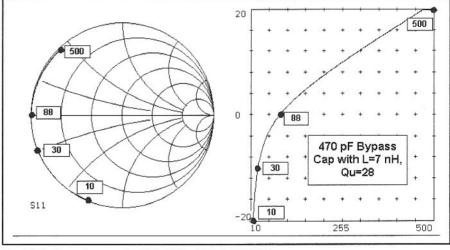
Fig 2.89—Impedance of a 470-pF bypass capacitor.
