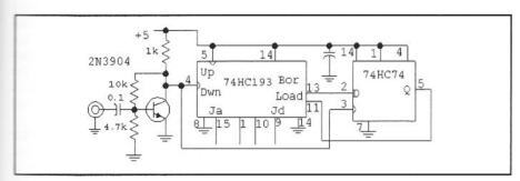
Fig 4.47—A simple programmable divider. See text.
