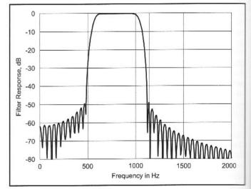
Fig 10.24—The out-of-band response for the 500-Hz filter of Fig 10.23. The design value for the side lobes was -50 dB.
