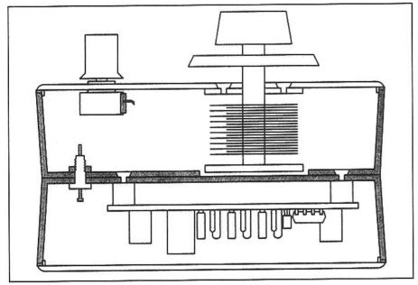
Fig 12.70—A Sleeping Bag Radio construction sketch.
