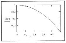
Fig 2.43—Power transfer related to reflection coefficient.
